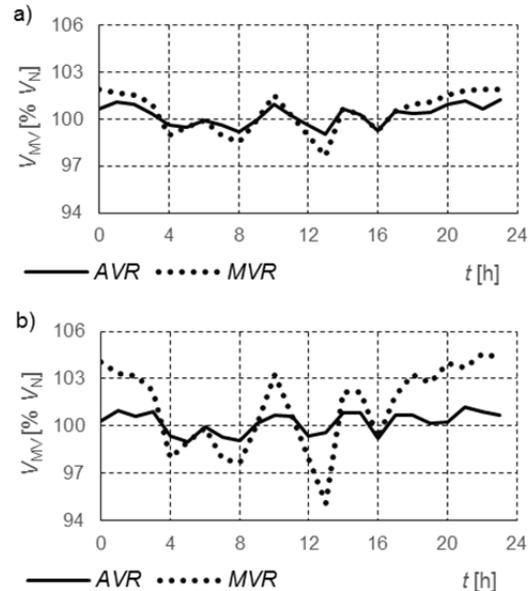
Fig.4. Voltage variations in the MV busbar of the HV/MV substation for *AVR* and *MVR* for the MV busbar 24 hour load profile and the 24 hour wind power generation profile with the *RMC* (a) and *VMC* (b)
