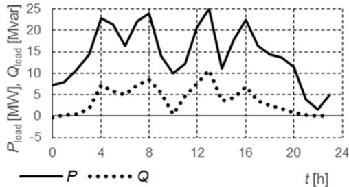
Fig.2. Daily load profile in the MV network
