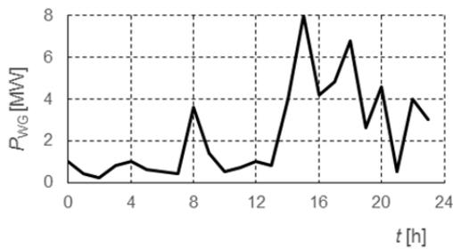
Fig.1. Daily active power generation profile of the wind farm
