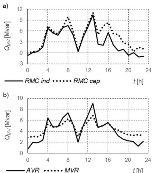
Fig.5. Variations of the reactive power feeding the MV power network of the analyzed power structure during the assumed 24 hour load profile changes and the wind power generation profile for: a) wind farm operating with the RMC ind and RMC cap; b) AVR and MVR in the substation and for the wind farm operating with the VMC
