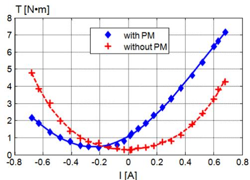
Fig.4. Clutching torque versus coil current  $T_C(I)$  – results of the measurements – for two type of magnetic excitation: + – only current carrying coil (without PM), ♦ – hybrid (with PM and current carrying coil) [8] at a temperature of 22 °C
