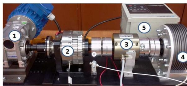
Fig.3. The test bench for the MR clutch: 1) gearmotor, 2) investigated MR clutch, 3) torquemeter, 4) load (brake), 5) inverter
