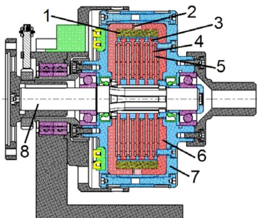
Fig.1. Axial section of magnetorheological clutch: 1 – coil of the clutch, 2 – permanent magnet, 3 – disc of driven member, 4 – MR fluid, 5 – disc of driving member, 6 – yoke of magnetic circuit, 7 – housing of the clutch, 8 – shaft of driving member
