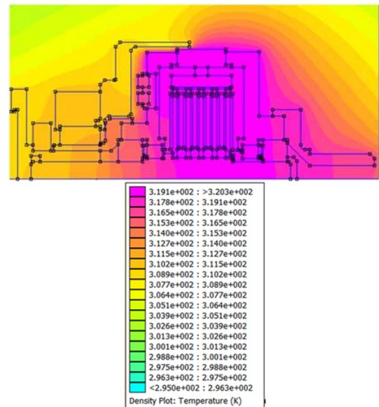
Fig.12. Result of thermal field analysis – temperature distribution field in MR clutch
