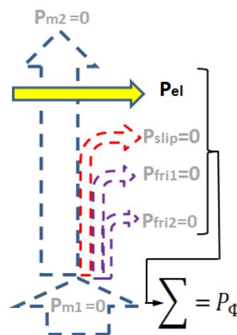
Fig.6. Source of the thermal power  $P_\Phi$  in the clutch during the electric heating
