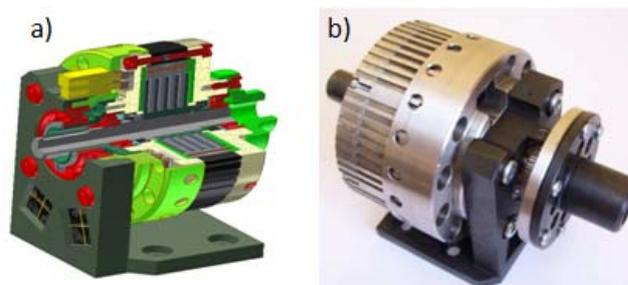
Fig.2. The magnetorheological multidisc clutch (MR clutch): a) 3D CAD model, b) the prototype [5], [8]
