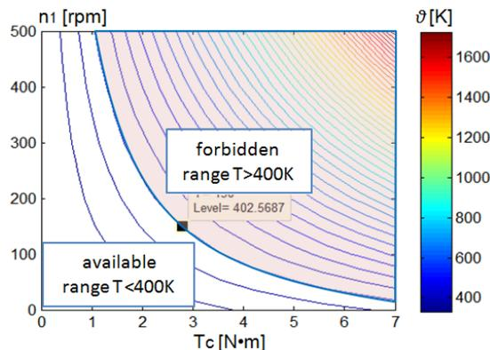
Fig.13. Available and not available operation range for MR clutch working in full slip state
