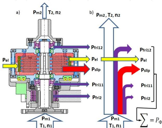
Fig.5. Diagram of power balance: a) the flow of power, b) sources of thermal power  $P_\Phi$  in the clutch
