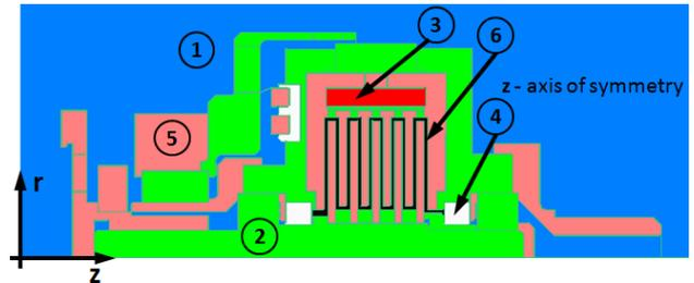
Fig.11. Axisymmetrical thermal model of the clutch: 1) air, 2) stainless nonmagnetic steel, 3) copper, 4) plastic, 5) carbon steel, 6) MR fluid
