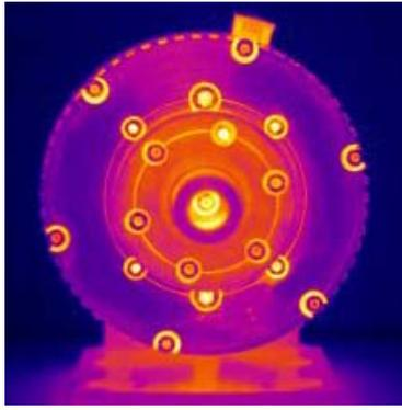
Fig.8. The image of the front surface of the MR clutch from the infrared camera recorded during the electric heating
