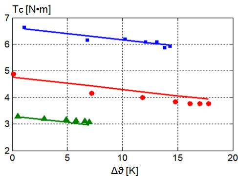
Fig.10. Results of measurements of influence of temperature  $\vartheta$  on clutching torque  $T_C$ , for three coil current:  $\blacktriangle$  –  $I=0.4$  A,  $\blacksquare$  –  $I=0.5$  A,  $\bullet$  –  $I=0.6$  A
