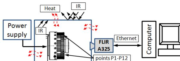
Fig.7. Schema of the thermal measurement system
