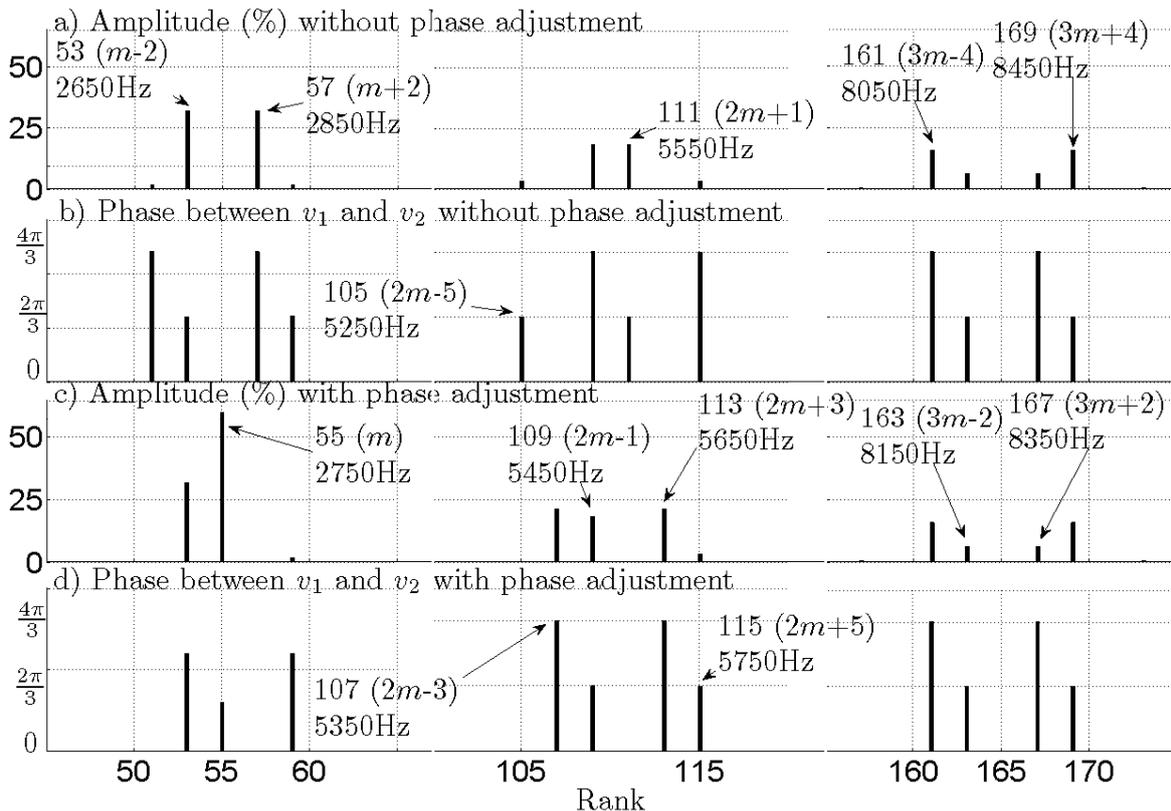
Fig. 3. Experimental  $v_1$  spectrum (in % of the fundamental) and phase difference with triangular carriers and  $m=55$  (The frequencies correspond to an operating point with  $f=50\text{Hz}$ )
