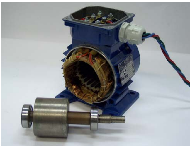
Fig. 1. The stator of the asynchronous motor with rotor made of infiltrated integrated core
