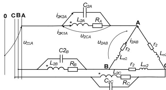
Fig. 2. Electric circuit consisting of secondary winding elements
