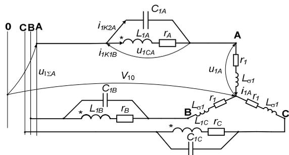
Fig. 1. Electric circuit consisting of primary winding elements
