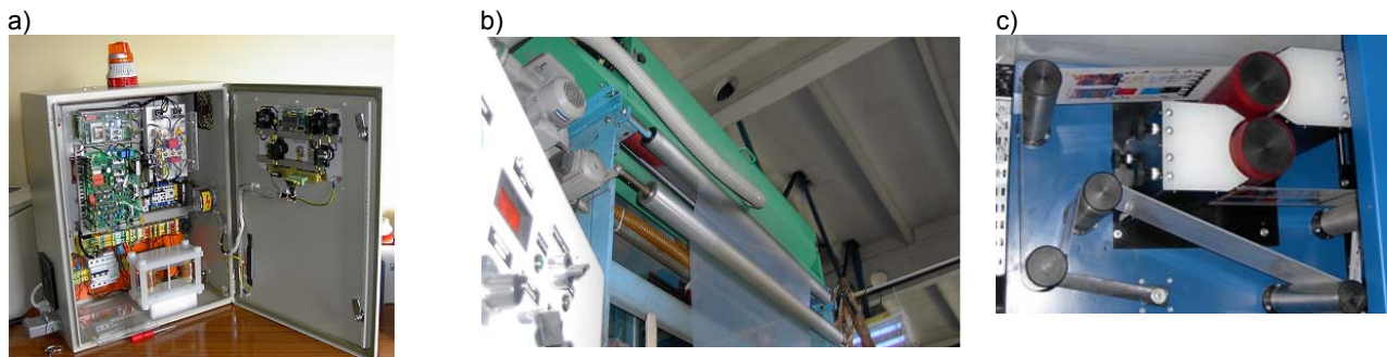
Fig. 6 Equipment for surface treatment of plastics by means of dielectric barrier (corona) discharge with generators (a) which were made on the basis of the author's documentation; processing of the film (b) and the adhesive label (c); elements of the lines was carried out in the Institute of Polymer Materials and Dyes Engineering (IMPIB) in Torun
