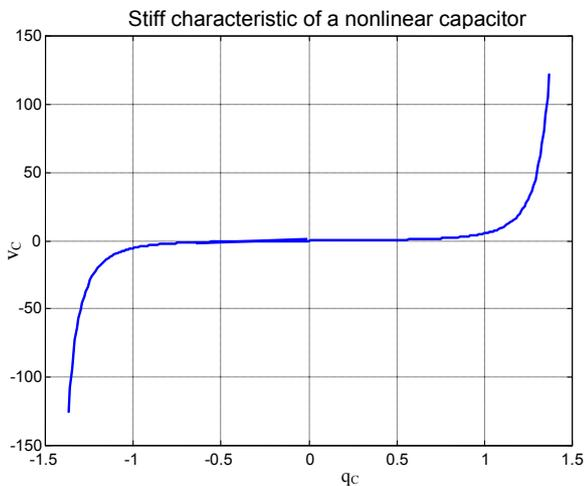
Fig.1. Characteristic of a nonlinear multilayer ceramic capacitor
