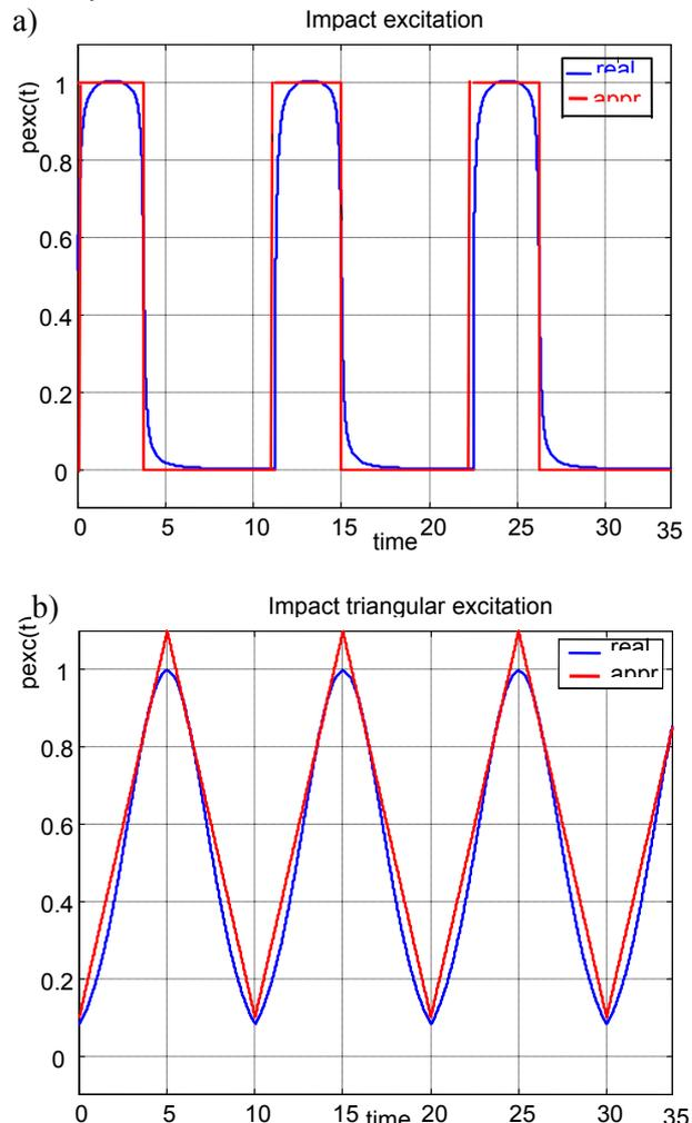
Fig.9. Two impact excitations: a) rectangular, b) triangular
