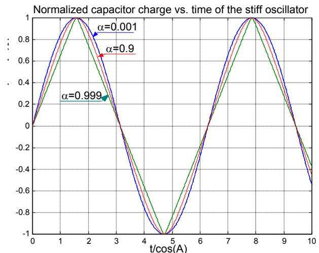
Fig.2.Changes in time of capacitor relative charge of the stiff oscillator for  $\alpha=\sin(A)$
