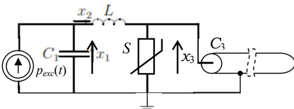
Fig.8. Overvoltage protection of power cable by surge arrester S
