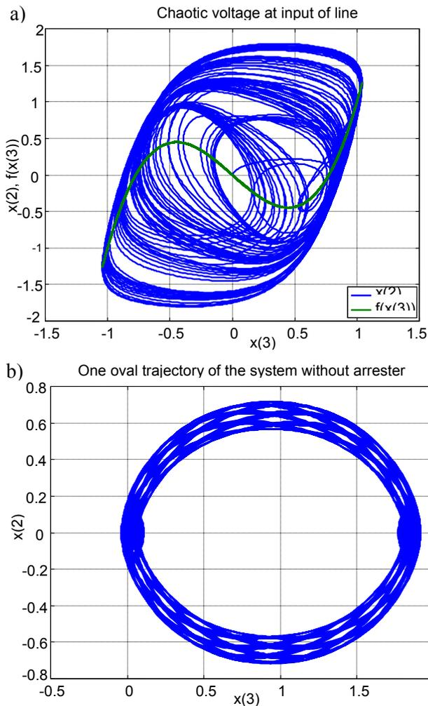
Fig. 10. Phase trajectory of the system: a) with surge arrester  $S$ , b) without surge arrester
