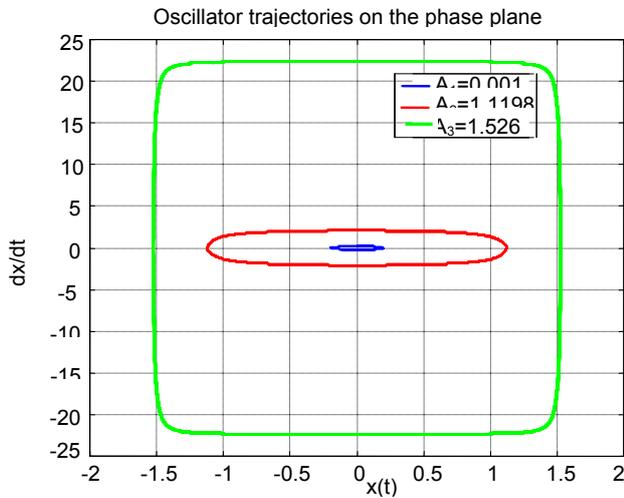
Fig.3. Steady state trajectories of stiff oscillator for different amplitudes (coordinates corresponding  $A_1$  are rescaled by  $10^3$ )
