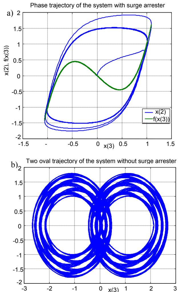
Fig. 11. The phase trajectory of the system: a) with surge arrester, b) without surge arrester
