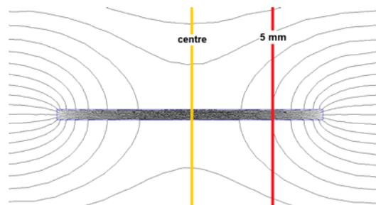
Fig.5. Normal component of  $H$  increases towards the edge of the sample (image not to scale, for conceptual illustration only)
