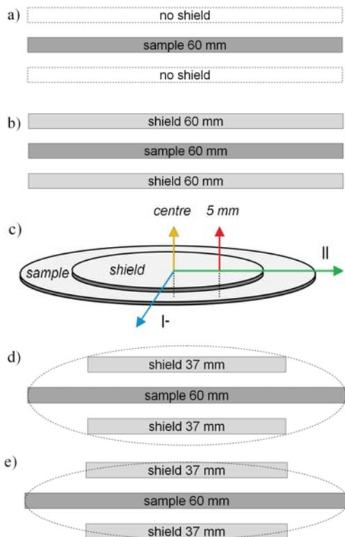
Fig.2. Modelled configurations: a) cross-section of a single circular sample, b) cross-section of a circular sample with two shields approximating a cylindrical structure, c) overview of a 3-layer approximated ellipsoid, d) and e) cross-section of a 3-layer approximated ellipsoid with alternative ellipse (drawings not to scale)
