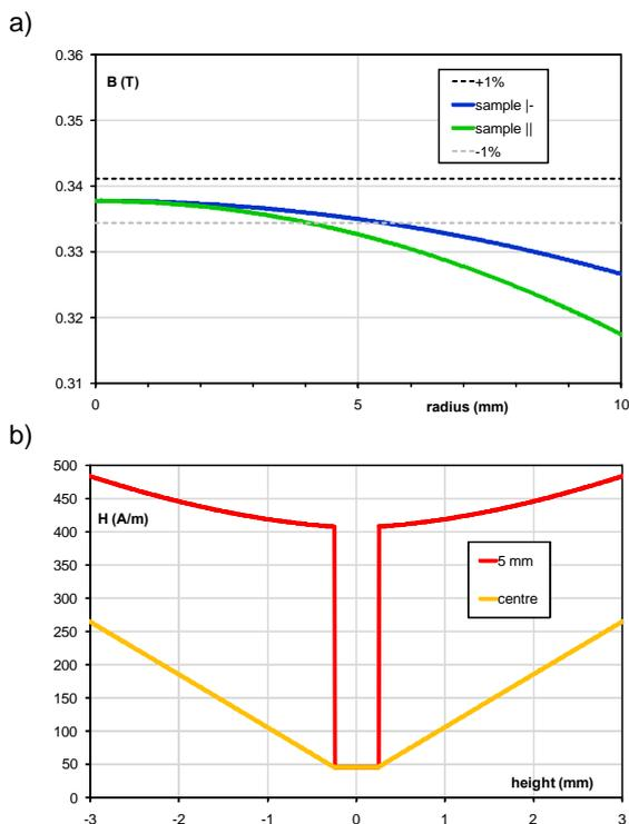
Fig.4. Distribution of  $B$  (a) and  $H$  (b) in a single lamination at low excitation, 1000 A-t (for the configuration shown in Fig. 2a)
