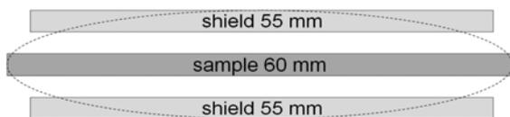
Fig.10. Cross-section of the optimised three-layer configuration (compare with Fig. 2d,e)
