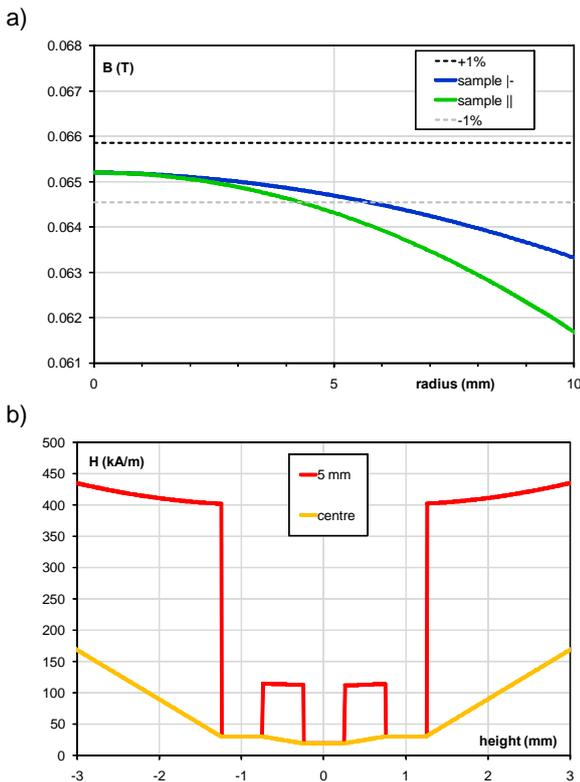
Fig.7. Distribution of  $B$  (a) and  $H$  (b) in the three-lamination system at low excitation, 1000 A-t (configuration from Fig. 2b)
