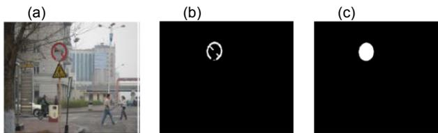
Fig.2. Segmentation process of partially occluded sign [33]
