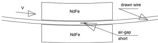
Fig. 7 Details of the scheme of Fig. 4 used for calculation with short air-gap
