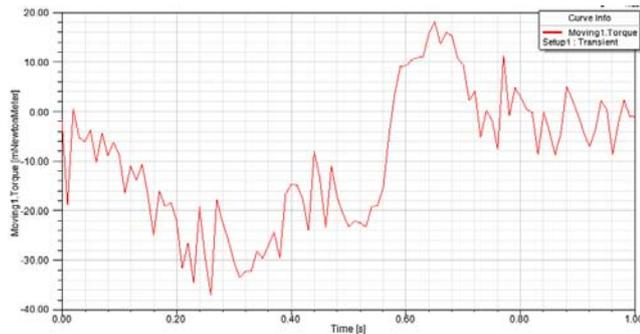
Fig. 8 Dependence of the torque from an angle of circle rotation for very short air-gap in the wire as in fig. 7
