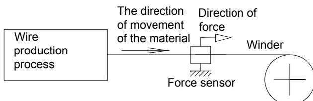
Fig. 1. Location of the sensor in a simplified schematic wire production.
