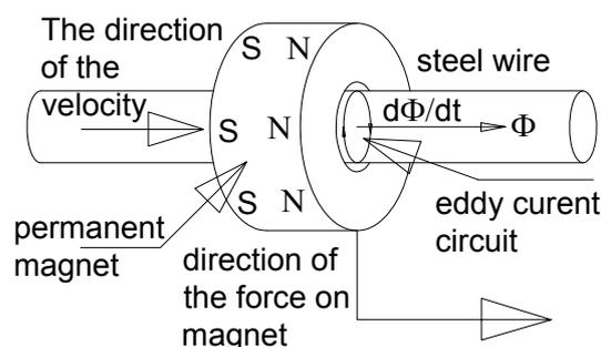
Fig.2 The principle of operation of the force sensor
