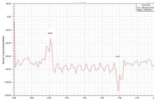
Fig. 6. Dependence of the torque from an angle of circle rotation . The simulated defect of the wire is located between the peaks on the diagram (Start-End).
