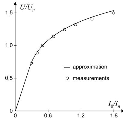
Fig. 1. No-load curve of induction motor [4]
