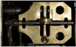
Fig. 2. Mechanism used in clocks in order to stabilize rotational speed – the example of variable moment of inertia  $J$ , dependent on angular velocity  $\omega$
