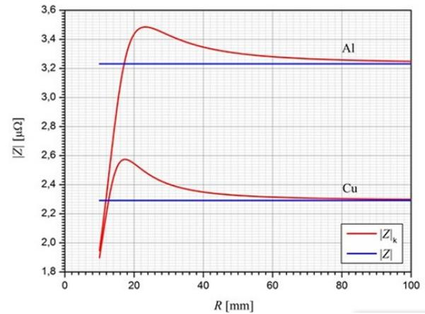
Fig.2a. Comparison of surface impedances calculated according to exact (2) and simplified formula (6) for Al and Cu screens; modules
