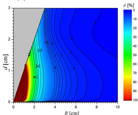
Fig.4. Dependence  $\delta$  as a function of screen curvature radius  $R$  and the screen thickness  $d$  for Al screen
