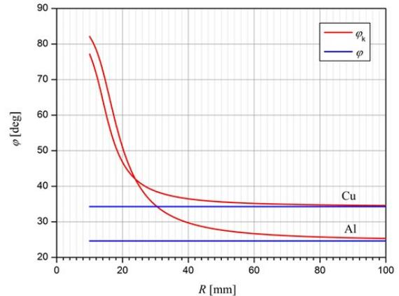
Fig.2b. Comparison of surface impedances calculated according to exact (2) and simplified formula (6) for Al and Cu screens; independent variables
