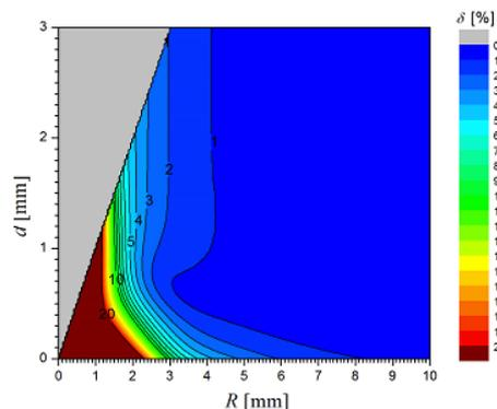
Fig.6. Dependence  $\delta$  as a function of screen curvature radius  $R$  and the screen thickness  $d$  for steel screen
