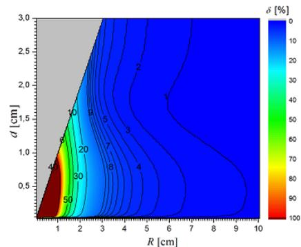
Fig.5. Dependence  $\delta$  as a function of screen curvature radius  $R$  and the screen thickness  $d$  for Cu screen
