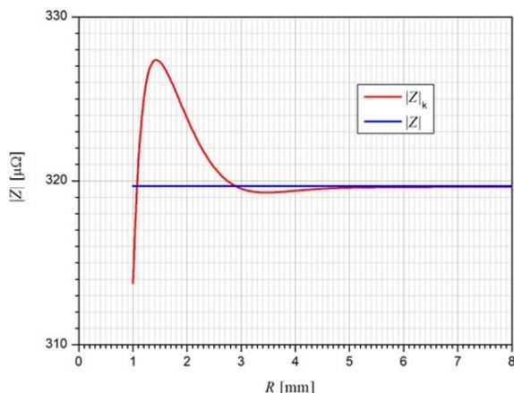
Fig.3a. Comparison of surface impedances calculated according to exact (2) and simplified formula (6) for a steel screen; modules
