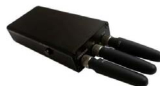
Figure 3: The GSM jammer used for the third experiment.
