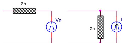
Fig.7. Equivalent parallel and series model of noise source
