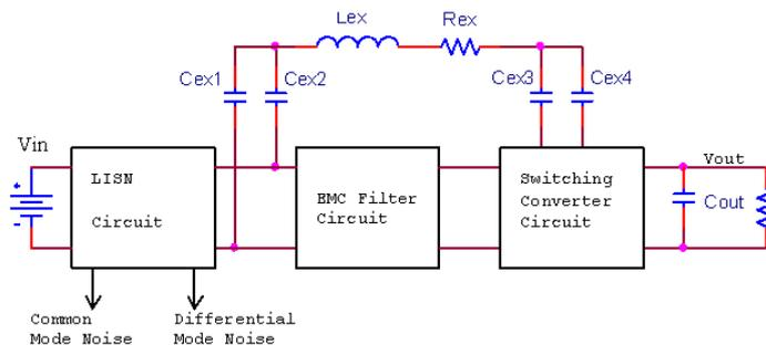
Fig.13. Final balanced arrangement of the proposed converter
