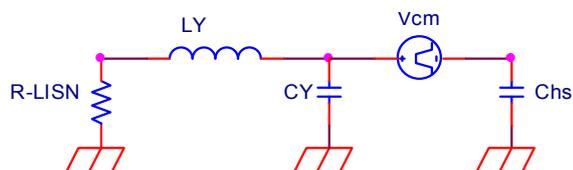
Fig.10. Equivalent noise model of the introduced converter
