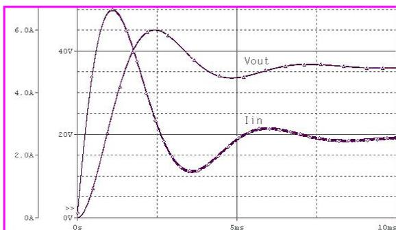
Fig.15. Converter output voltage with its input current
