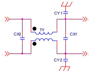
Fig.8. EMI filter circuit used here
