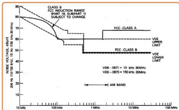
Fig.9. FCC and VDE standards limit for conducted noise
