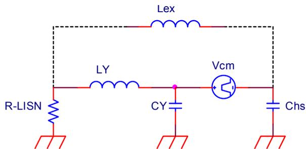
Fig.11. Balance circuit of the converter noise model
