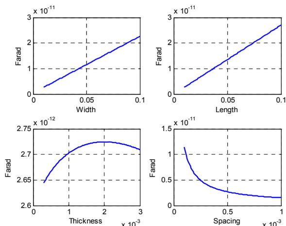
Fig.4. Parasitic capacitor curves on the basis of  $w$ ,  $l$ ,  $t$  and  $h$  items
