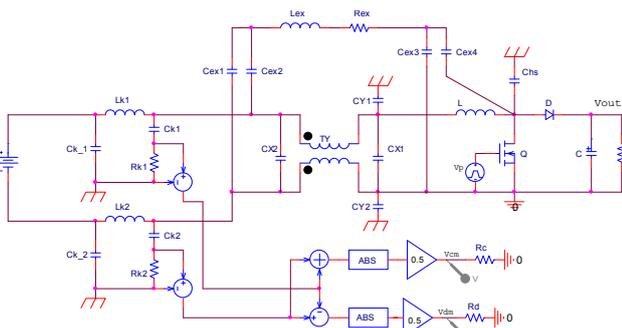
Fig.14. Simulated converter final circuit
