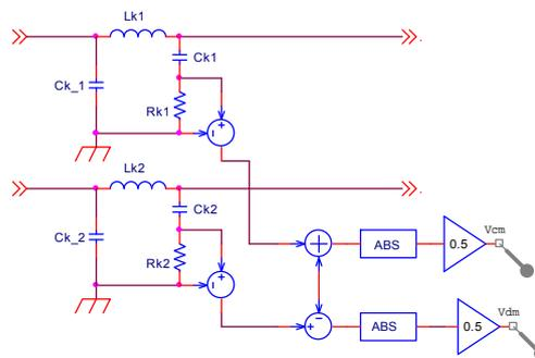
Fig.6. LISN equivalent circuit used to extract the CM and DM noise
