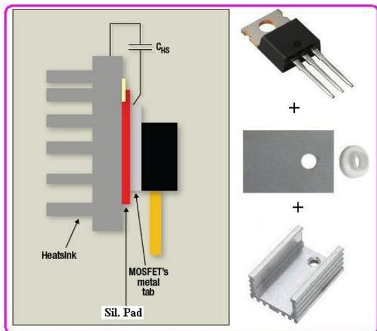
Fig.3. Switch supplement and its parasitic capacitor
