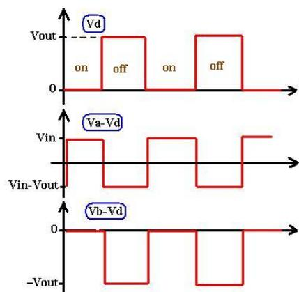
Fig.2. Nodes voltage of the boost voltage shown in Fig.1
