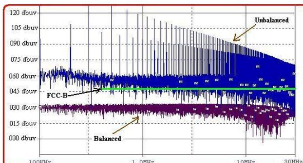
Fig.16. CM noise in the both balanced and unbalanced cases
