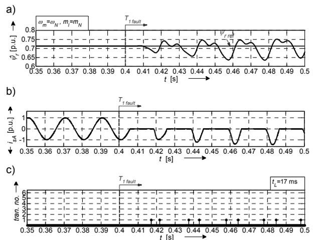
Fig.10. Reference  $\psi_{r\ ref}$  and absolute value of the estimated rotor flux  $\hat{\psi}_r$  (a) current in the faulty inverter phase  $i_{sa}$  (b) and output signal of the fault diagnostic system  $tran. no.$  (c) in case of  $T_1$  fault
