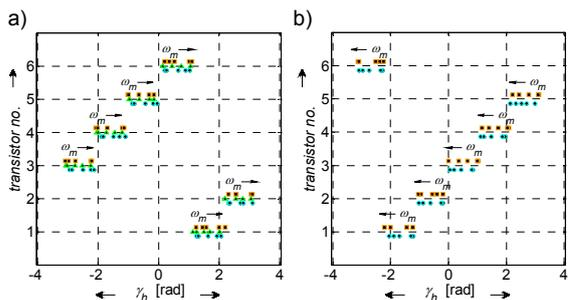
Fig.9. Registered values of the angle  $\gamma_h$  during the inverter transistor faults at the angular motor speed:  $\omega_m > 0$  (a) and  $\omega_m < 0$  (b)
