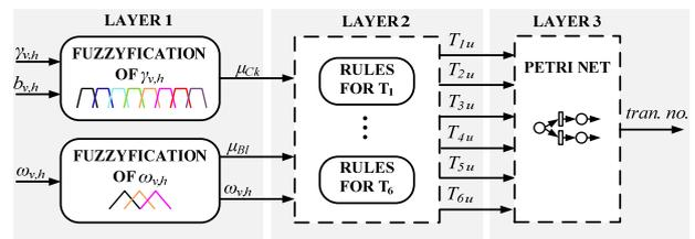
Fig.6. Block diagram of the fault symptoms integration stage of the diagnostic procedure
