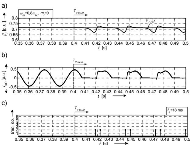
Fig.11. Reference  $\psi_r$  and absolute value of the estimated rotor flux  $\psi_r$ , (a) current in the faulty inverter phase  $i_{sc}$  (b) and output signal of the fault diagnostic system  $tran. no.$  (c) in case of  $T_2$  fault
