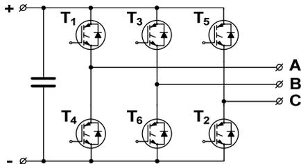
Fig.1. Two-level three-phase voltage inverter topology
