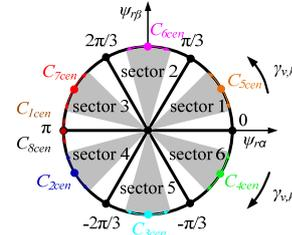
Fig.5. Relationship between sectors of the  $\alpha$ - $\beta$  plane and  $C_k$  functions
