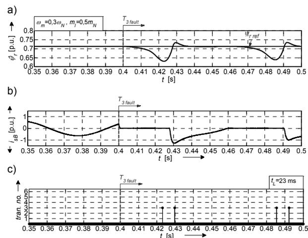
Fig.12. Reference  $\psi_r$  and absolute value of the estimated rotor flux  $\psi_r$ , (a) current in the faulty inverter phase  $i_{sB}$  (b) and output signal of the fault diagnostic system  $tran. no.$  (c) in case of  $T_3$  fault
