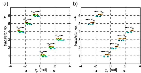
Fig.8. Registered values of the angle  $\gamma_v$  during the inverter transistor faults at the angular motor speed:  $\omega_m > 0$  (a) and  $\omega_m < 0$  (b)
