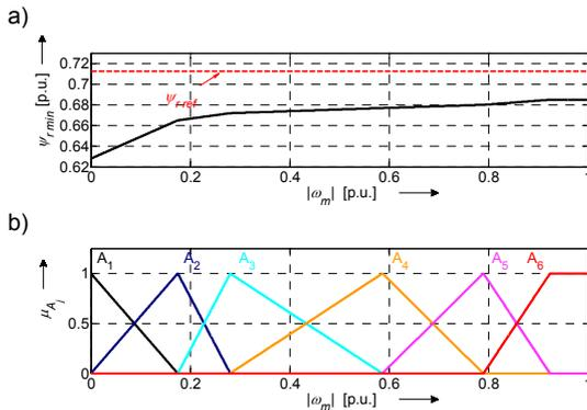
Fig.3. Function  $\psi_{r \min}(|\omega_m|)$  (a) and membership functions  $A_j$  (b)
