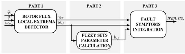
Fig.2. Sequential diagnostic system scheme
