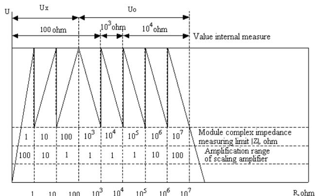
Fig. 3. Measurement limit of module complex impedance  $|Z|$  by an immittance meter E7-25
