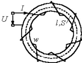
Fig. 1. A coil with toroidal ferromagnetic core
