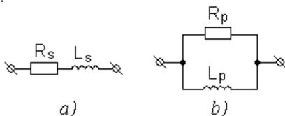
Fig. 2. Equivalent inductance coil circuits
