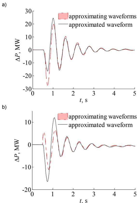
Fig. 2. Waveforms of the instantaneous power deviation in unit no 11 in Łaziska Power Plant in case of pulse (a) and step (b) disturbance of amplitude  $\Delta V_{ref} = -5\% V_{ref0}$
