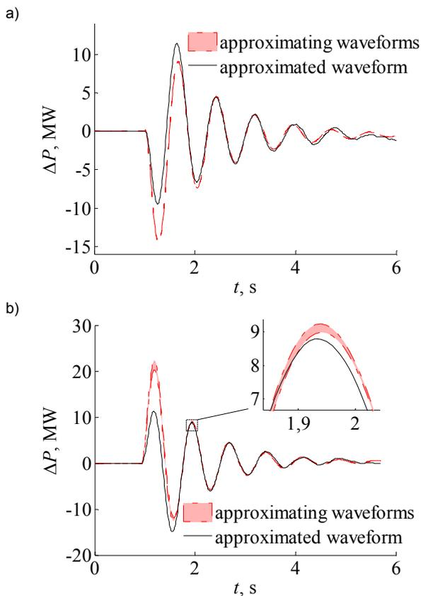
Fig.3. Waveforms of the instantaneous power deviation in unit no 11 in Łaziska Power Plant in case of step disturbance of amplitude  $\Delta V_{ref} = -3\% V_{ref0}$  (a) and  $\Delta V_{ref} = 3\% V_{ref0}$  (b)
