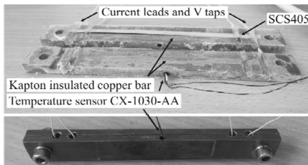
Fig. 7. Experimental setup – HTS tape probe
