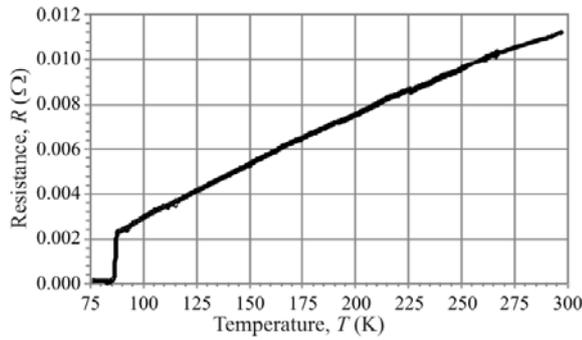
Fig. 8. Measured temperature-dependent resistance of the 4-mm-wide SCS4050 tape (length of tape: 10 cm)
