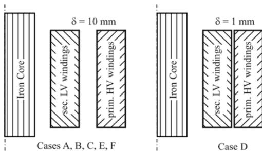
Fig. 5. Air-gap width in the transformers
