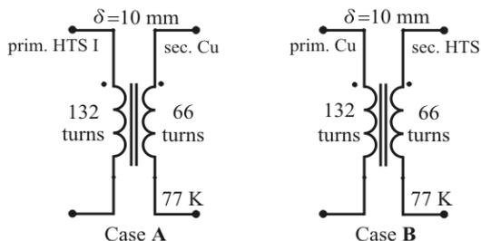
Fig. 2. Diagrams of transformers with windings made of copper wire and SCS4050 tape
