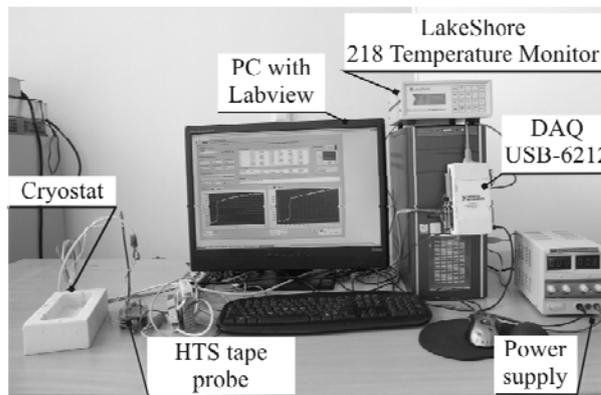
Fig. 6. Experimental setup for measurement the resistance of HTS tape
