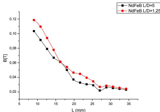
Graph 3. Comparison of the magnetic induction B distribution with respect to the line y for NdFeB L/D=5 and L/D=1,25.
