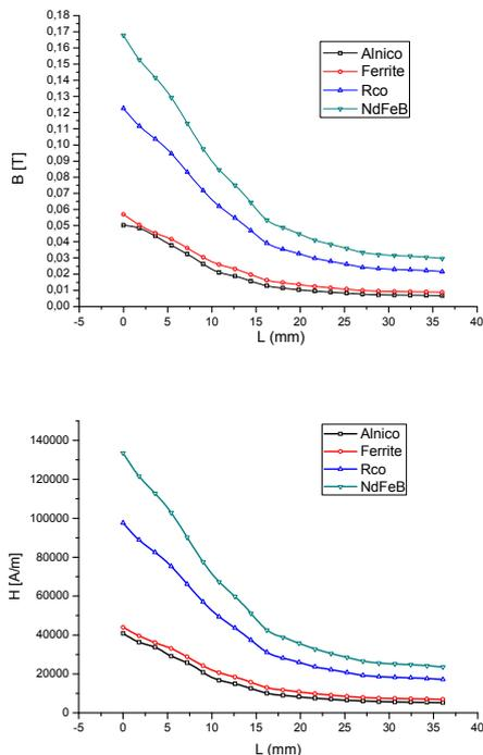
Graph 1. Values of the magnetic field induction B and magnetic field intensity H in the models examined; L/D=5.
