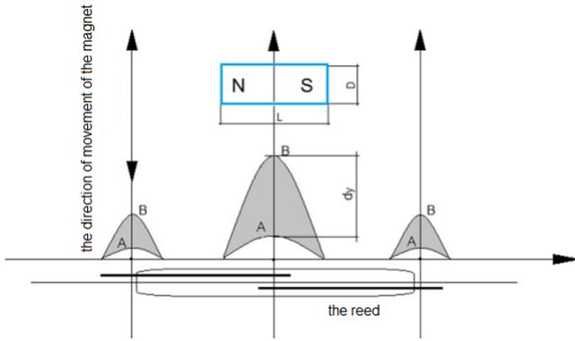
Fig. 2. Actuating the reed switch by means of a permanent magnet in a system with a parallel movement of the magnet with respect to the longitudinal axis of the reed switch.
