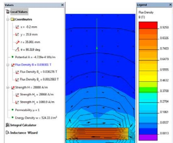
Fig. 5. The example for N38 - region of the magnetic field analysis with respect to the lateral symmetrical y of the model, D=4mm (magnet diameter), L=20mm (length), L/D=5 and the temperature 26,5°C. [source: developed by the authors]
