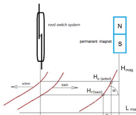
Fig. 1. Influence of the reed switch parameters and of the magnetic field gradient on the value of the reverse shift  $dy$ .
