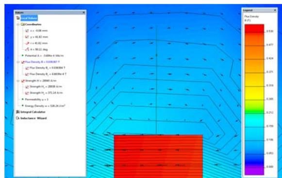
Fig. 6. Computations and distribution of the magnetic induction B and of magnetic field intensity H obtained with respect to the line y for NdFeB; the dimensions are D = 8mm, L = 10 mm (L/D=1,25), the temperature is 26,5°C.
