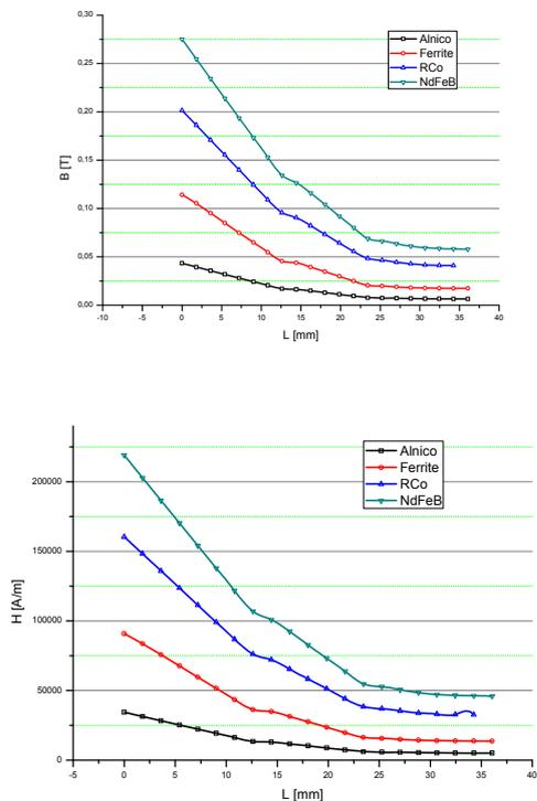
Graph 2. Values of the magnetic field induction B and magnetic field intensity H in the models examined; L/D=1,25.
