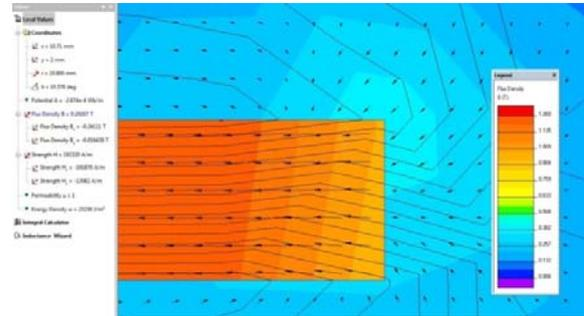
Fig. 4. Analysis of magnetic induction B in the region of one of the poles of magnet N38 [source: developed by the authors]
