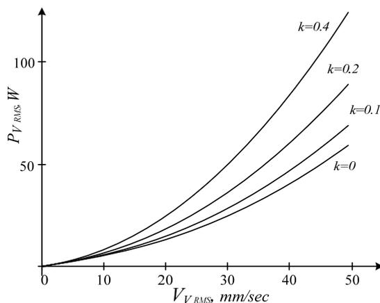
Fig. 3 Dependence of vibration power RMS value on vibration velocity RMS value under stator windings faults
