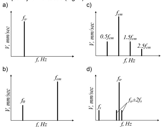
Fig. 2 Typical form of IM vibration velocity spectra for most common fault types: imbalance (a), rotor eccentricity (b), stator faults (c), rotor broken bars (d)
