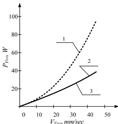
Fig. 1 Vibration power RMS value dependence on vibration velocity RMS value for the defects: 1 – stator damage, 2 – rotor broken bars, 3 – rotor imbalance
