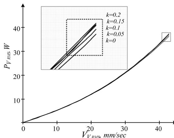
Fig. 5 Dependence of vibration power RMS value on vibration velocity RMS value in the presence of rotor broken bars
