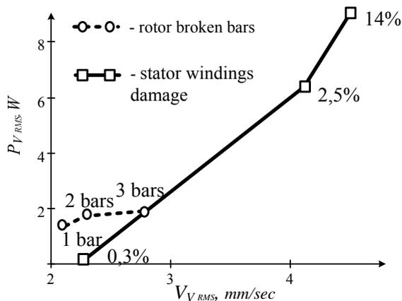
Fig. 6 Dependence of vibration power RMS value on vibration velocity RMS value when stator are damaged and rotor broken bars
