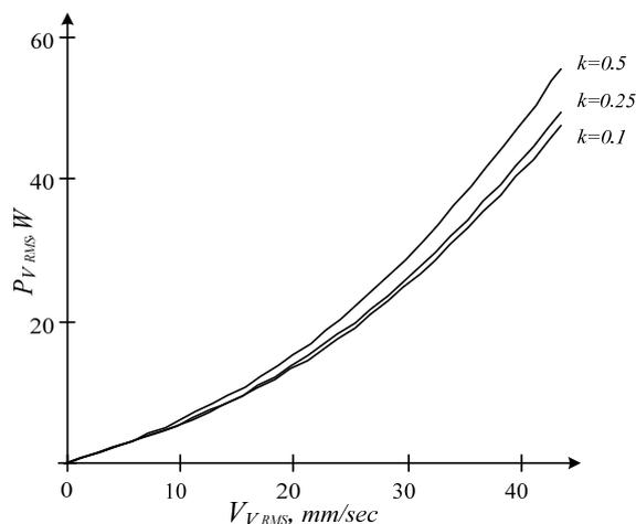
Fig. 4 Dependence of vibration power RMS value on vibration velocity RMS value in the presence of rotor eccentricity
