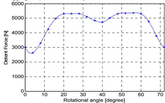
Fig. 14. Detent force of single-layer AFPMSM
