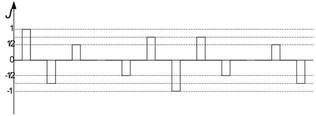
Fig.5. Distribution of current density in the coil sides along the periphery of AFPMSM with double-layer windings at the moment which corresponds to  $t=0$
