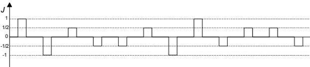
Fig.3. Distribution of current density in coil sides along the periphery of AFPMSM with single-layer stator windings at the moment which corresponds to  $t=0$
