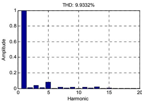
Fig. 10. Back EMF harmonic components of single-layer AFPMSM
