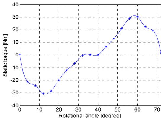
Fig. 17. Static torque of double-layer AFPMSM
