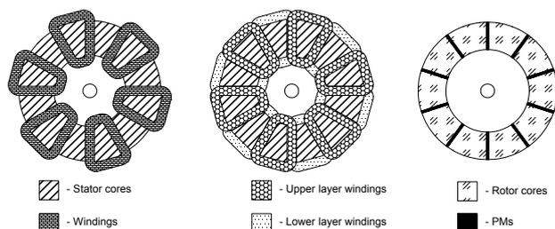
Fig. 1. Topologies of AFPMSMs
