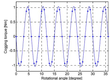
Fig. 13. Cogging torque of double-layer AFPMSM
