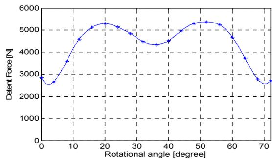
Fig. 15. Detent force of double-layer AFPMSM
