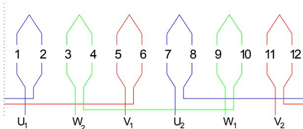
Fig.2. Connections between coils of single-layer stator windings
