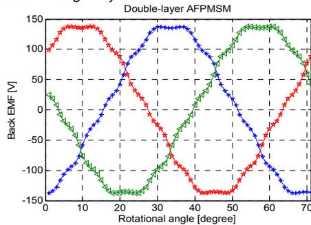
Fig. 9. Back EMF of double-layer AFPMSM
