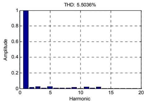
Fig. 11. Back EMF harmonic components of double-layer AFPMSM
