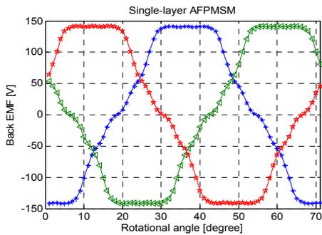
Fig. 8. Back EMF of single-layer AFPMSM
