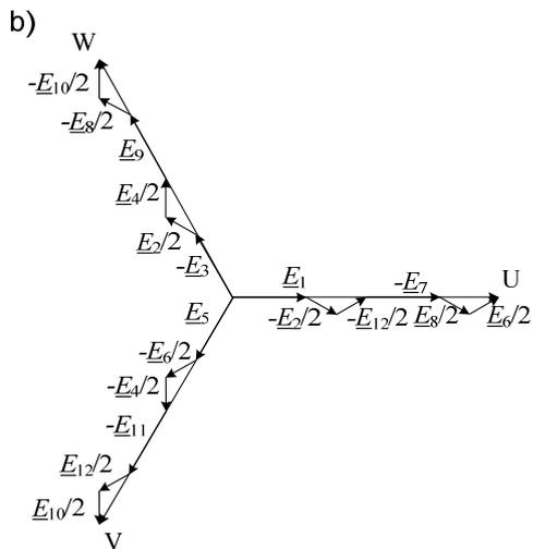
Fig. 7. Vector sum of slots EMFs per phase for a) single-layer winding and b) double-layer winding ( $U$ ,  $V$  and  $W$  are phase back EMFs)
