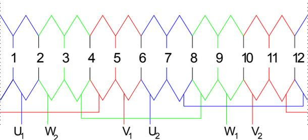
Fig.4. Connections between coils of double-layer stator windings
