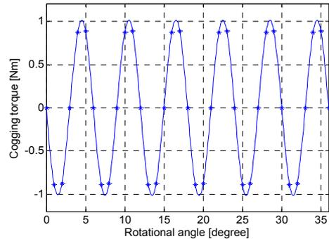
Fig. 12. Cogging torque of single-layer AFPMSM
