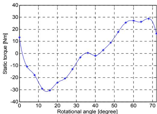
Fig. 16. Static torque of single-layer AFPMSM
