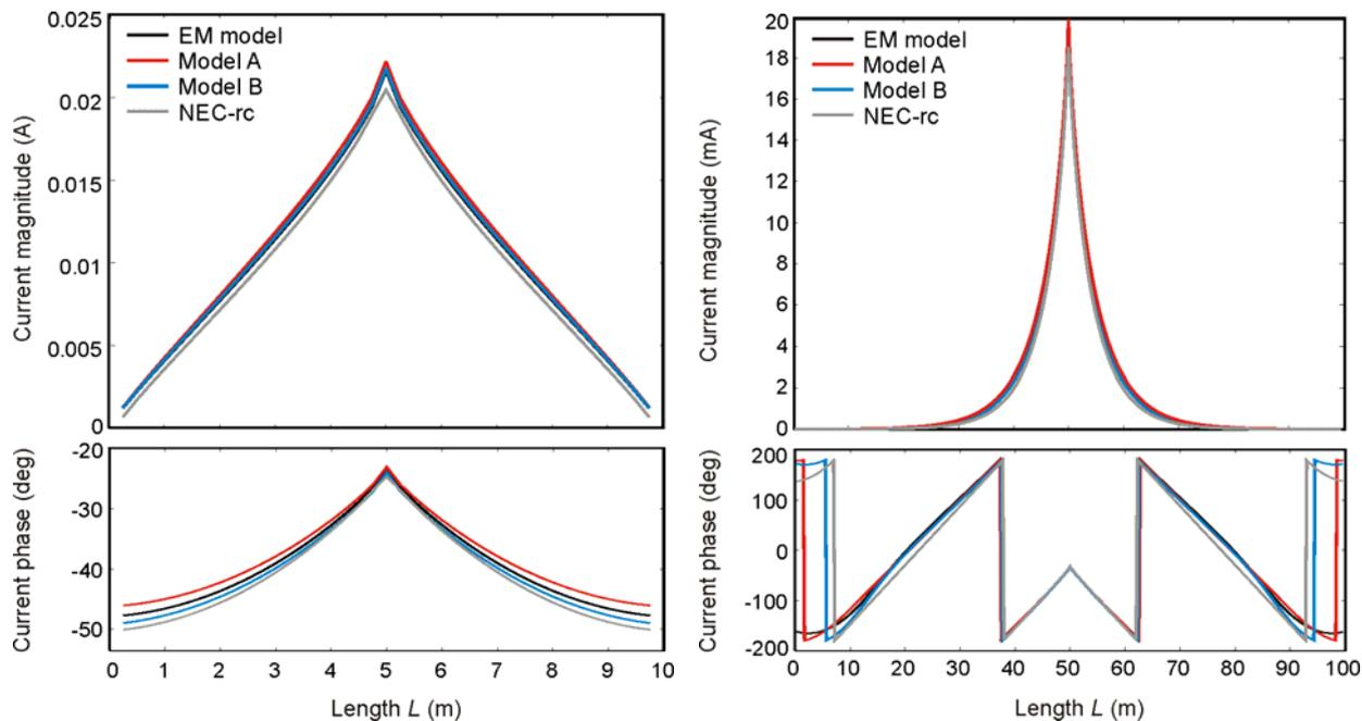
Fig.2. Current magnitude and phase along a 10-m conductor (left) and 100-m conductor (right) at 1 MHz obtained by different models ( $D = 1$  m,  $\sigma = 0.01$  S/m)
