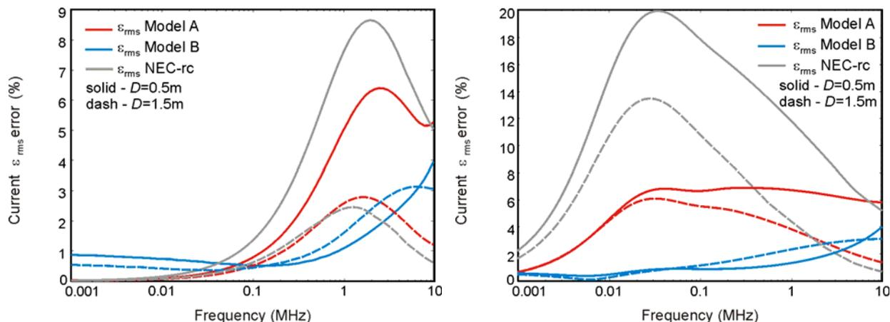
Fig.5. Influence of the soil conductivity on the  $\epsilon_{rms}$  error obtained for  $\sigma = 0.001$  S/m and  $\sigma = 0.1$  S/m ( $L = 10$ -m - left) and ( $L = 10$ -m - right)
