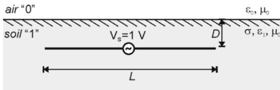
Fig. 1. A centre fed horizontal conductor in homogeneous lossy soil
