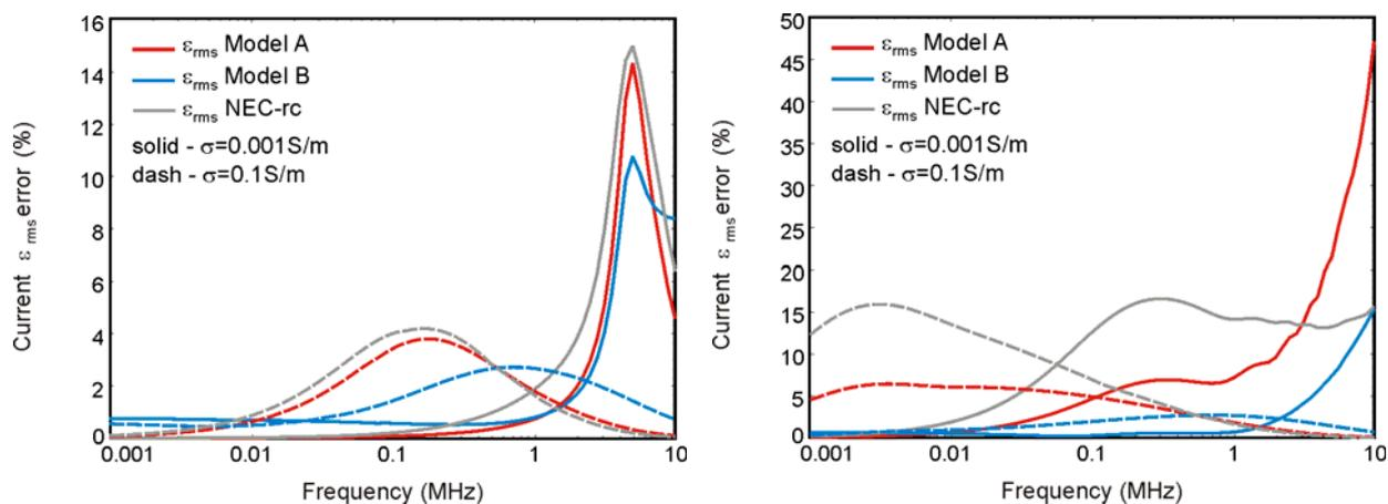
Fig.4. Influence of the conductor depth on the  $\epsilon_{rms}$  error obtained for  $D = 0.5$  m and  $D = 1.5$  m ( $L = 10$ -m - left) and ( $L = 10$ -m - right)
