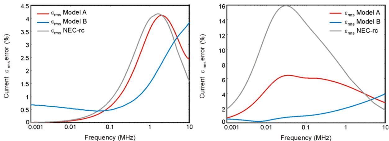
Fig.3. Current rms error obtained by approximate models A and B: conductor length  $L = 10$ -m, depth  $D = 1$  m,  $\sigma = 0.01$  S/m (left), and  $L = 100$ -m,  $D = 1$  m,  $\sigma = 0.01$  S/m (right)
