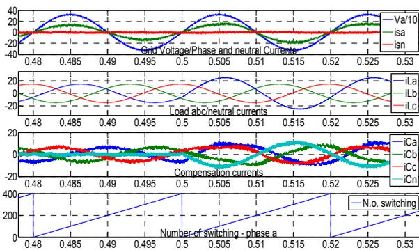
Fig. 6 SAPH with linear current control; Load 2 - operation performance, from the top: phase A grid voltage  $V_a$  and current  $i_{sa}$  (THD=3,9%) and neutral current  $i_{sn}$ , load currents with neutral current, compensation currents, number of switching in SAPH phase A per grid voltage period (20ms)
