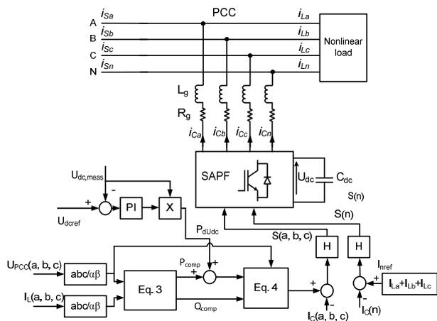
Fig. 2 Instantaneous power theory based control scheme for SAPF
