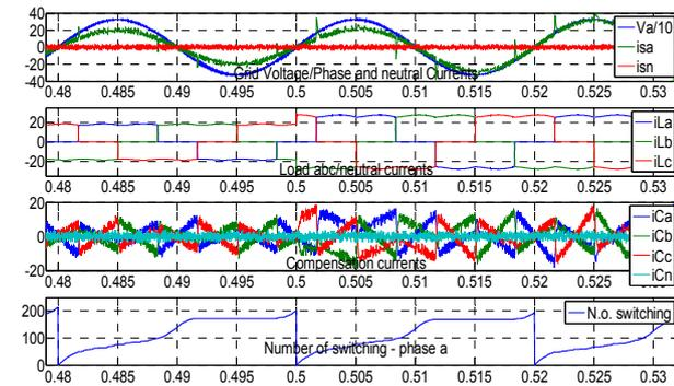
Fig. 8 SAPH with instantaneous power theory based control; Load 1 - operation performance, from the top: phase A grid voltage  $V_a$  and current  $i_{sa}$  (THD=9,5%), load currents, compensation currents, number of switching in SAPH phase A per grid voltage period (20ms)
