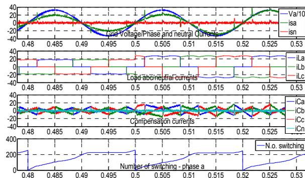
Fig. 10 SAPH with FS-MPC; Load 1 - operation performance, from the top: phase A grid voltage  $V_a$  and current  $i_{sa}$  (THD( $i_{sa}$ )=9,5%), load currents, compensation currents, number of switching in SAPH phase A per grid voltage period (20ms)
