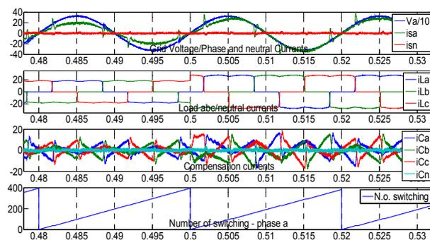
Fig. 9 SAPH with linear current control; Load 1 - operation performance, from the top: phase A grid voltage  $V_a$  and current  $i_{sa}$  (THD( $i_{sa}$ )=17,5%), load currents, compensation number of switching in SAPH phase A per grid voltage period (20ms)
