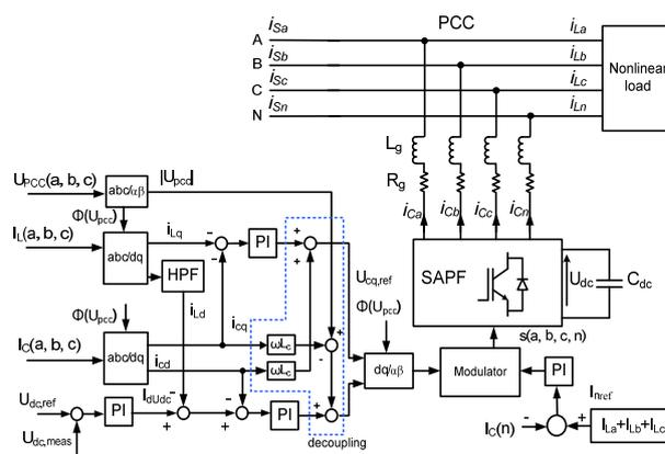
Fig. 3 Linear current control scheme for SAPF
