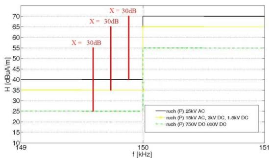
Fig. 5 Presentation of forecasted differences in values of the same magnetic field measured below (BW = 200Hz) and above (BW = 9000 Hz) border frequency 150 kHz with usage of different BWs (peak detector).
