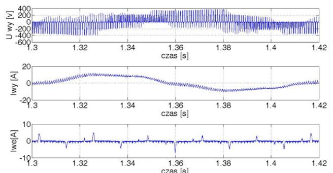
Fig.2 Exemplary curves registered in a drive system with an inverter and an asynchronous motor (from the top: output voltage (phase) of inverter-motor, output current (phase) of inverter-motor; input current (phase) of an inverter)
