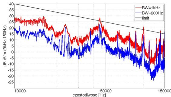
Fig.19 Comparison of disturbances generated by a tram for two values of BW.
