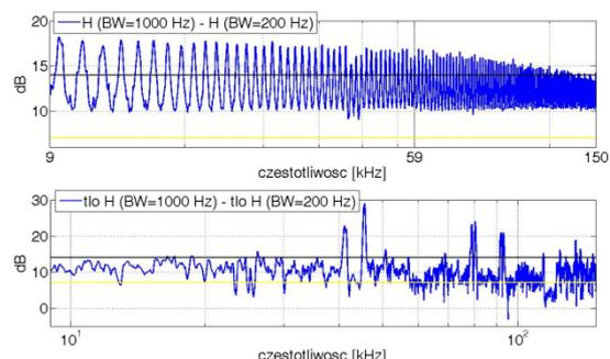
Fig.12 Comparison of differences of chopper and background noise values of disturbances at two BWs of a receiver (correction factors for totally coherent signals of about 14 dB and incoherent of about 7 dB were marked).
