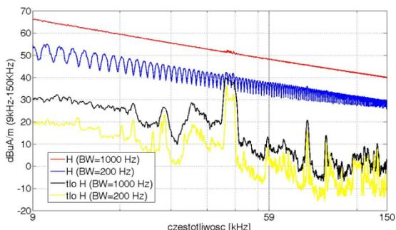
Fig.11 Results of registration of disturbances generated by a chopper-motor system and a background noise in the band 9 kHz-150 kHz at two BWs.
