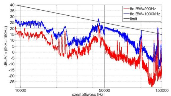
Fig.18 Comparison of a background noise at measurement site registered for two values of BW.
