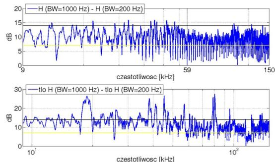
Fig.7 Comparison of differences between the values of disturbances of an inverter and a background noise measured at two BWs of a receiver (correction factors were marked for signals that are completely coherent, around 14 dB and incoherent around 7 dB).
