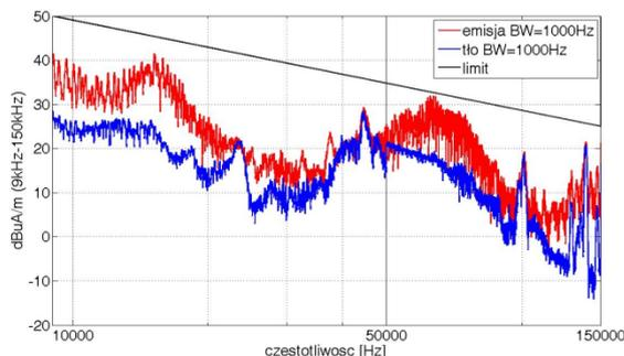
Fig. 21 Comparison of disturbances generated by a tram in motion with a background, for 1000Hz measurement bandwidth.
