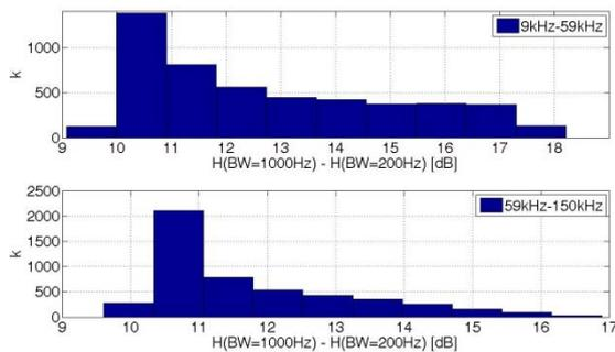
Fig. 14 Histograms showing a difference in values of disturbances from a chopper-motor system registered for various BWs in the range of frequencies 9 kHz-59 kHz and 59kHz-150 kHz [Lack of test points removed from the assessment of results due to the close value of background and device disturbances-values that are always higher than 4 dB]
