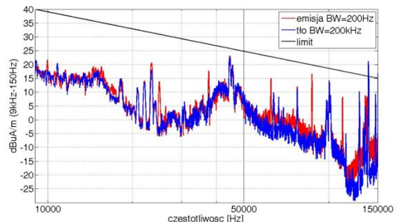
Fig.17 Results of registration of disturbances from a tram under measurements and a background noise for a BW 200 Hz.
