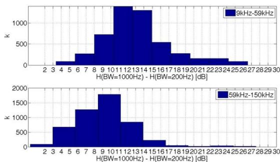
Fig.8a Histograms showing a difference in values of background noise at the measuring place of an inverter-motor system registered for the frequency ranges 9 kHz-59 kHz and 59 kHz-150 kHz (k-number of test points).
