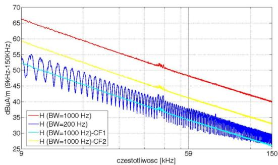
Fig. 13 Results of registration of disturbances from a chopper-motor system in the frequency range 9 kHz-150 kHz at two BWs and with application of corrections CF1, CF2 for values measured by 1000 Hz BW.
