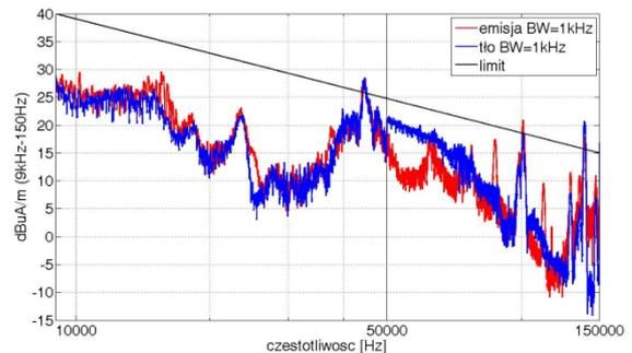
Fig.16 Results of registration of disturbances from the tram under measurements and a background noise for a BW 1kHz.
