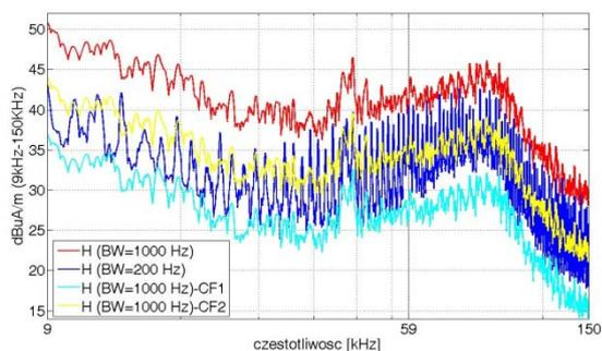
Fig. 9 Results of registration of disturbances from an inverter-motor system in a range of frequencies 9 kHz- 150 kHz at two BWs with application of CF1, CF2 corrections for the values measured by 1000 Hz bandwidth.
