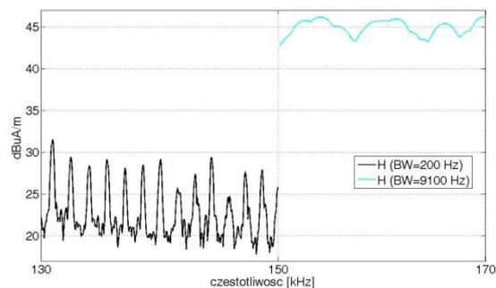
Fig.10 Results of registration of disturbances from an inverter-motor system in the range of 150 kHz frequency at two BWs.
