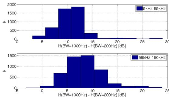
Fig. 14a Histograms showing a difference in values of a background noise at the measuring place of a chopper-motor system registered for various bandwidths in the range of frequencies 9 kHz-59 kHz and 59 kHz-150 kHz.
