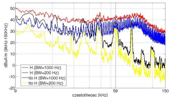
Fig.6 Results of registration of disturbances generated by an inverter-motor system and a background noise in a band 9 kHz-150 kHz at two BWs.
