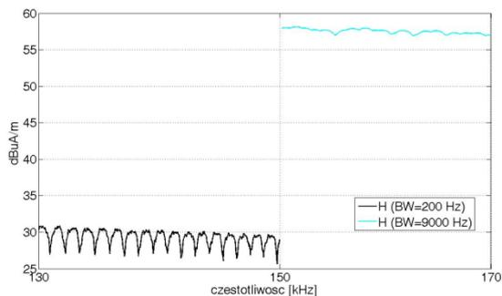
Fig. 15 Results of registration of disturbances from a chopper-motor system around frequency of 150 kHz at two BWs.
