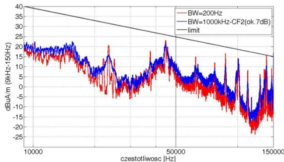
Fig.20 Comparison of disturbances generated by a tram for two values of BW, with application of a correction factor CF2 (around 7dB).
