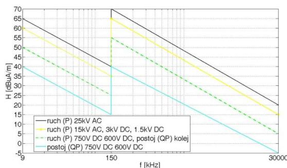
Fig 3. Limits of admissible disturbances for a magnetic component in the frequency range 9kHz- 30 MHz specified in the standard [2] during a slow moving test ( P- peak detector)) and a during stop (QP- quasi peak detector)).
