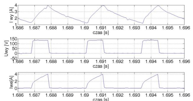
Fig.1 Exemplary curves registered in a drive system with a chopper (from the top: chopper output current-motor current, chopper output voltage- motor voltage; chopper input current).
