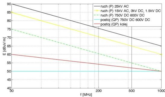
Fig.4 Limits of admissible levels of disturbances for the electric component in the frequency range 30 MHz-1 GHz defined in the standard [2] during a slow moving test (P-peak detector) and during a stationary test (QP-quasi-peak detector) [apart from measurements of magnetic component disturbances, one performs measurements of vertical and horizontal electric component disturbances].
