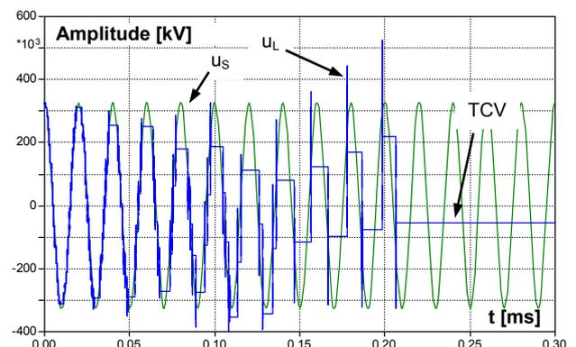
Fig. 2 Very Fast Transient process;  $u_s$  – disconnector source side voltage,  $u_L$  – disconnector load side voltage, TCV – Trapped Charge Voltage
