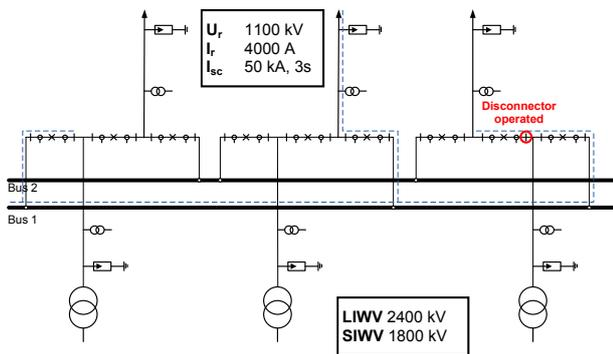
Fig. 5 Single line diagram of an exemplary UHV GIS substation in one and half circuit breaker arrangement with the calculation path indicated
