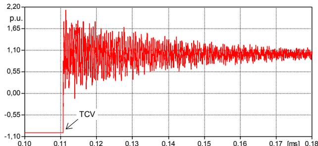
Fig. 7 VFTO waveform for disconnector load side; contact speed 3.0 m/s, TCV 99% = -1 p.u. (3 m/s), VFTO = 2.14 p.u.
