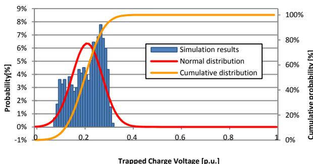
Fig. 3 TCV calculated for TD1 set-up for opening operation, with contact speed 0.39 m/s and nominal voltage 1100 kV
