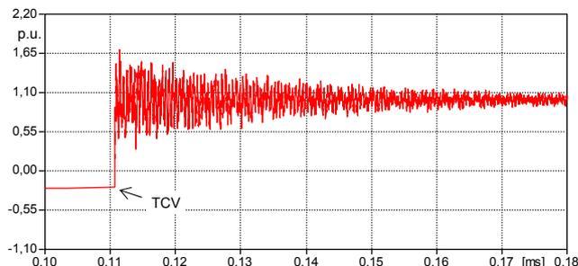
Fig. 6 VFTO waveform for disconnector load side; contact speed 0.1 m/s, TCV 99% = 0.24 p.u. (0.1 m/s), VFTO = 1.70 p.u.
