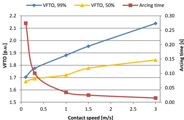
Fig. 8 VFTO and sparking time for different 99% TCV associated with different speeds of disconnecter moving contact (0.1-3.0 m/s)
