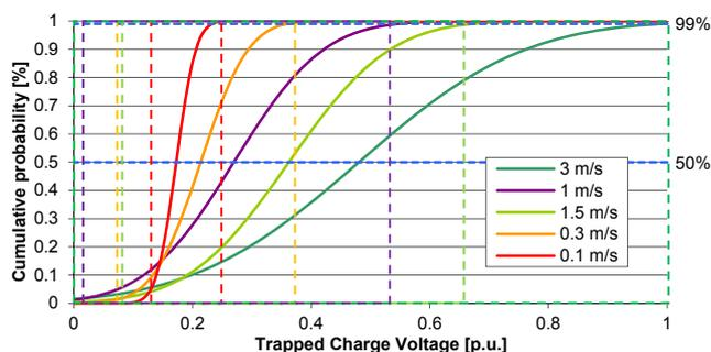
Fig. 4 Cumulative distributions of TCV for different contact speeds
