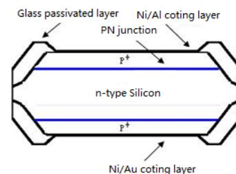
Fig. 2 The cross-section view of SMBJ
