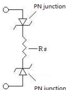
Fig. 3 Equivalent circuit schematics of SMBJ under DC
