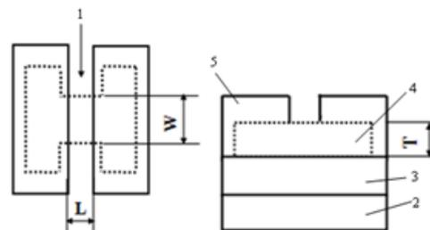
Fig. 1. Schematic view of a typical SCB
