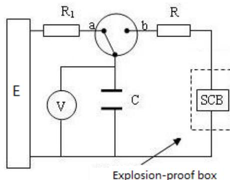
Fig. 4 Electrostatic experiments principle circle schematics
