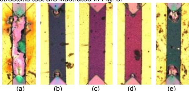
Fig.5 the damage situation of SCB bridge region under different test conditions
