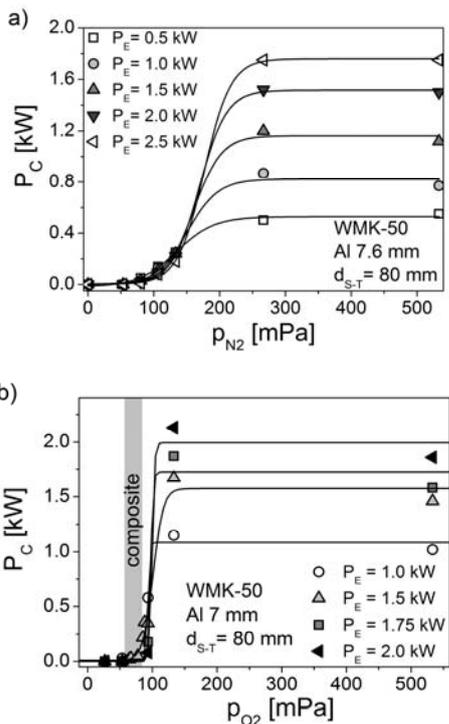
Fig.2. Circulating power  $P_C$  versus reactive gas partial pressure for magnetron sputtering of Al target: a) sputtering in  $N_2+Ar$  gas mixture b) sputtering in  $O_2+Ar$  gas mixture
