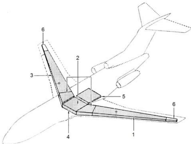
Fig. 3. Fuel tank configuration of a commercial aircraft (Boeing 727). 1 – wing tank No 1, CWT No 2 (three sections), 3 – wing tank No 3, 4 – integral tank, 5 – aft auxiliary tank, 6 – vent surge tank [2].
