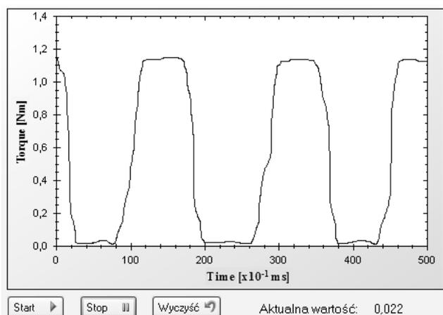
Fig. 9. Torque characteristic of stepper motor measured using FAST technique with external load
