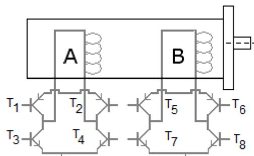
Fig. 6. Bipolar control mode of stepper motor
