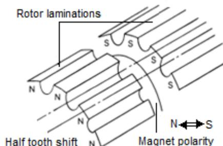
Fig. 1. A view of hybrid stepper motor rotor
