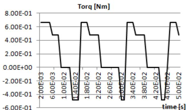
Fig. 8. Torque characteristic of stepper motor simulated using FEM method without external motor load
