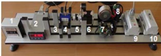
Fig. 4. The laboratory kit with FAST technology torque sensor DFM22-2.5 .where: 1 – unipolar/bipolar control mode switch, 2 – torque gauge MD100M, 3 – gear drive system, 4 – DFM 22-2.5 torque sensor , 5 – clutch, 6 – stepper motor, 7 – motor controller, 8, 10 – voltage power supply, 9 – modul that defines the motor trajectory (PC connected)
