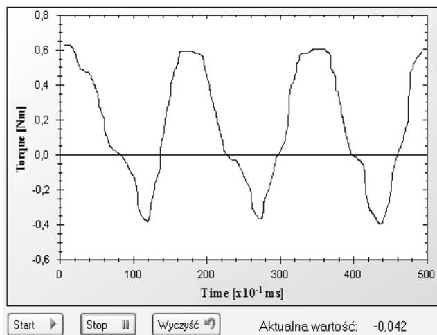
Fig. 7. Torque characteristic of stepper motor measured using FAST technique without external motor load
