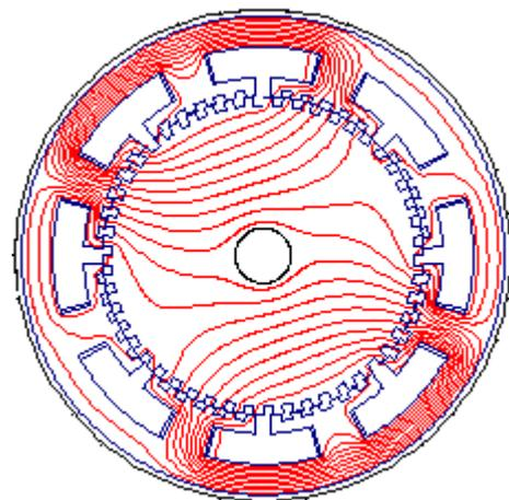
Fig. 3. Electromagnetic field distribution of the hybrid stepper motor
