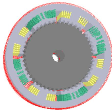
Fig. 2. Full 3D mesh of the hybrid stepper motor model
