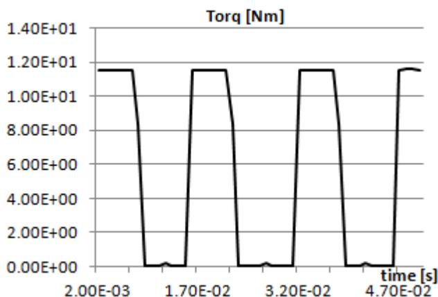
Fig. 10. Torque characteristic of stepper motor simulated using FEM method with external load
