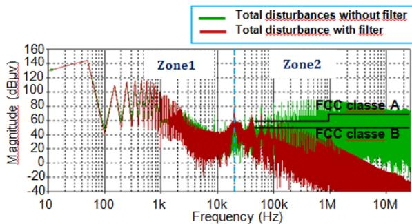
Fig. 12. Total disturbances with and without filter spectrum corresponding to the association rectifier-chopper
