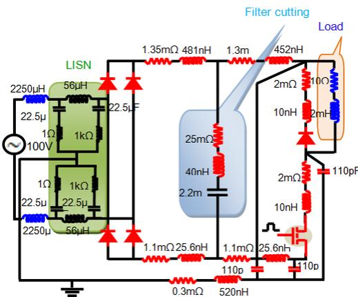
Fig.2. Rectifier-Chopper association - Assembly scheme
