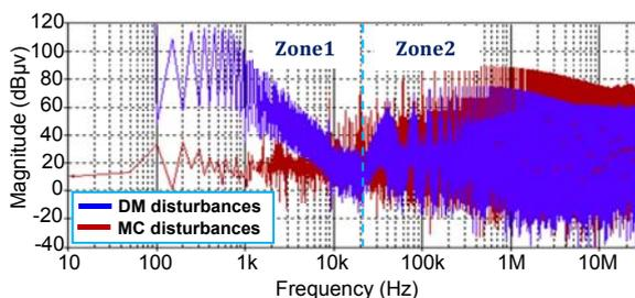
Fig. 7. Differential and common mode disturbances
