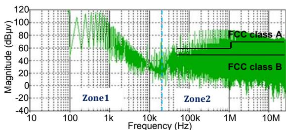
Fig. 6. Total disturbances spectrum due to the rectifier-chopper association
