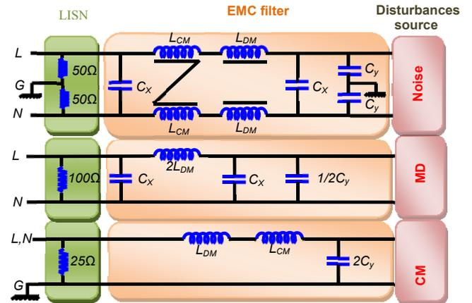
Fig. 11. Typical topology of an EMC filter used in the CM and DM modes [7], [12], [13], [16]
