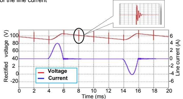
Fig. 4. Temporal variations of the bridge rectifier output voltage and of the line current
