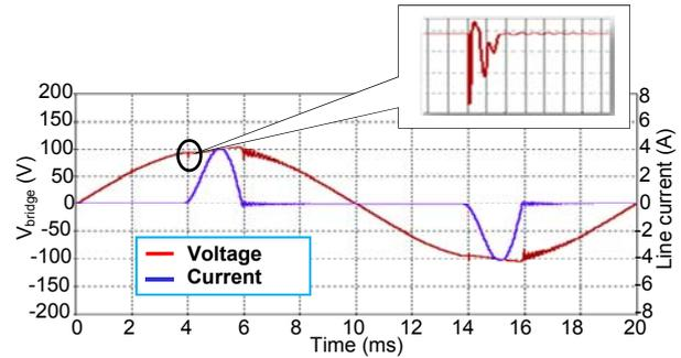
Fig.3. Temporal variations of the bridge rectifier input voltage and of the line current
