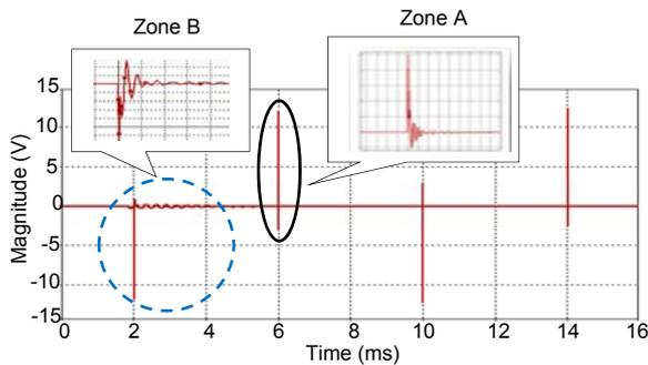
Fig. 5. LISN equivalent resistance terminal voltages
