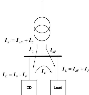
Figure 3. Optimal non-pulsed mode at asymmetrical voltage
