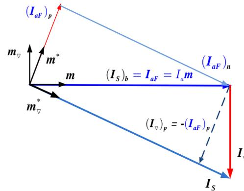
Figure 2. Addition of the unbalanced current to the active current in order to eliminate pulsation
