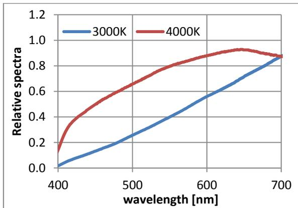
Fig. 4. Spectral power distribution of halogen reference lamps.
