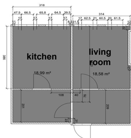
Fig. 1. Ground plan of full scale laboratory rooms with control rooms.
