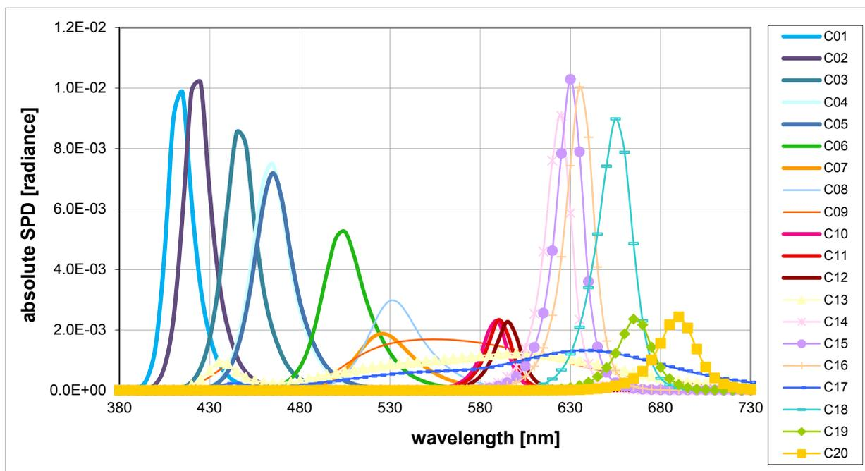
Fig. 5. SPD of LEDs built-in into the tuneable LED light source.
