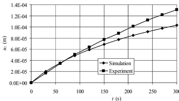
Fig. 8. Time evolution of the axial displacement ( $I_{\text{eff}} = 1 \text{ A}$ ,  $f = 2210 \text{ Hz}$ )
