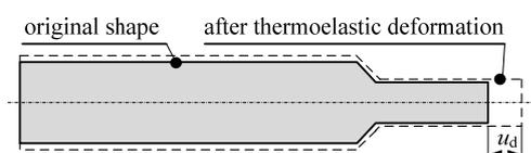
Fig. 2. Dilatation element **2** before and after deformation
