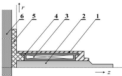
Fig. 1. The basic arrangement of the device **1** – Teflon shell, **2** – dilatation element, **3** – field coil, **4** – fixing frame, **5** – Teflon front, **6** – stiff wall
