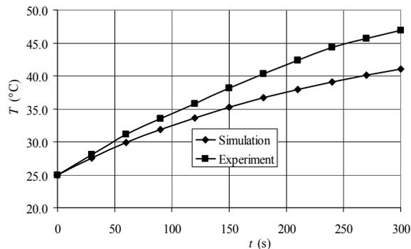
Fig. 7. Time evolution of the temperature ( $I_{\text{eff}} = 1 \text{ A}$ ,  $f = 2210 \text{ Hz}$ )
