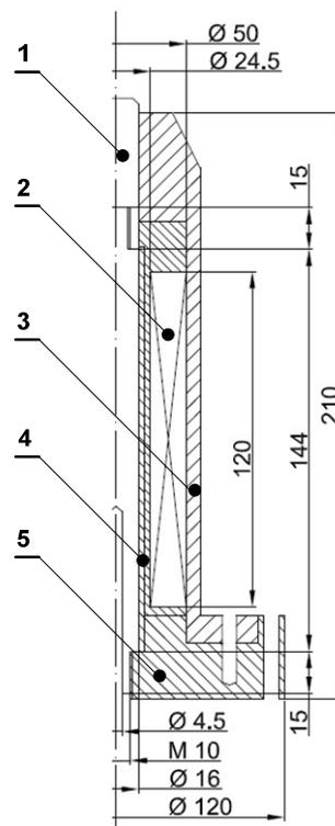
Fig. 4. Arrangement of the tested actuator (dimensions in mm) 1–brass dilatation element, 2–field coil, 3–nylon shell, 4–ceramic tube, 5–nylon bottom
