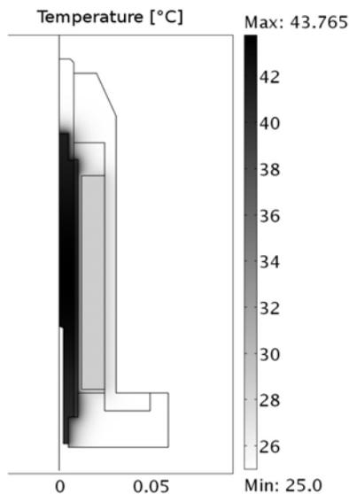
Fig. 5. Distribution of temperature in the system ( $t = 300 \text{ s}$ ,  $I_{\text{eff}} = 1 \text{ A}$ ,  $f = 2210 \text{ Hz}$ )
