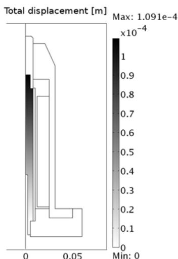
Fig. 6. Distribution of displacements in the dilatation element ( $t = 300 \text{ s}$ ,  $I_{\text{eff}} = 1 \text{ A}$ ,  $f = 2210 \text{ Hz}$ )
