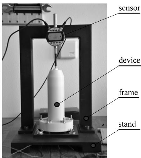
Fig. 3. Experimental stand with the device
