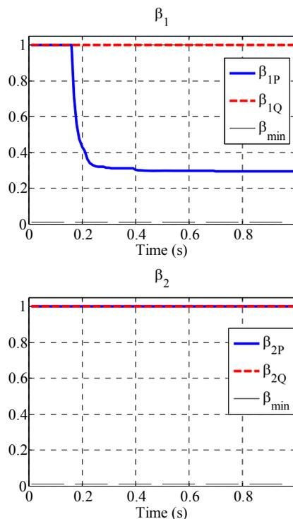
Fig.8 Beta coefficients (18) for the microgrid in Fig. 6 before and after the load step (synchronized with the step)
