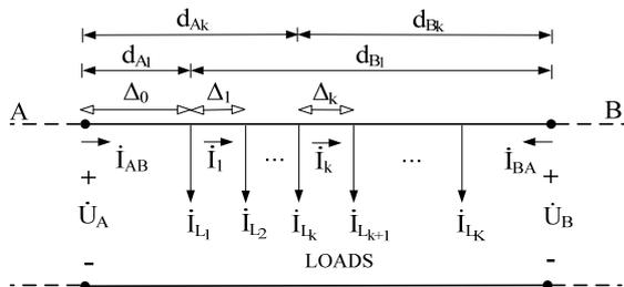
Fig. 2 – Representation of the distribution line between two active nodes A and B
