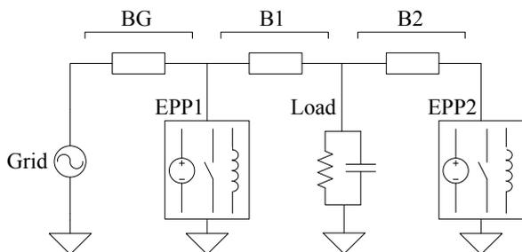
Fig.6 Reduced microgrid implemented in the real-time platform
