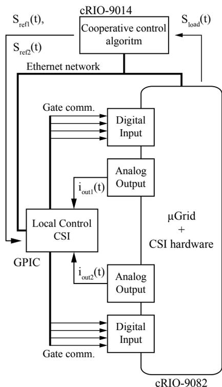
Fig.7 Architecture of the real-time platform
