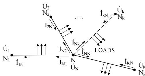
Fig. 3 – Representation of a grid section converging in node N
