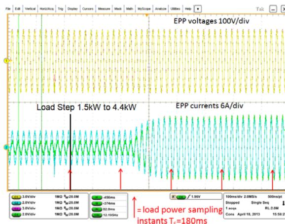
Fig.10 Voltages and currents of the EPPs as generated by the analog output modules of the real-time simulator
