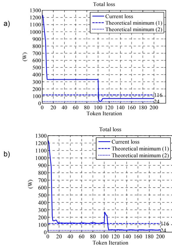
Fig.5 Distribution loss in the microgrid of Fig. 4, with EPPs driven by Cooperative Control
