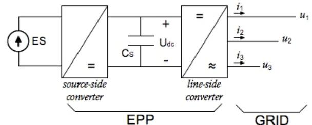
Fig. 1 - General structure of a distributed energy resource (DER) equipped with electronic power processor (EPP)
