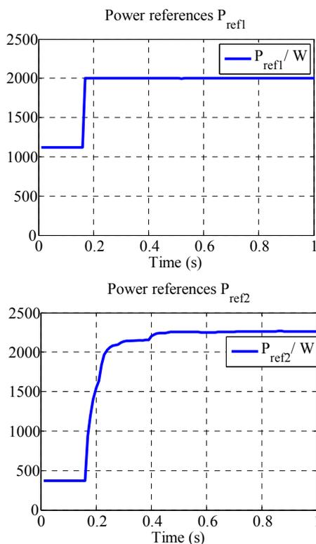
Fig.9 Active power injected by the EPPs in the microgrid of Fig. 6 before and after the load step (synchronized with the step)
