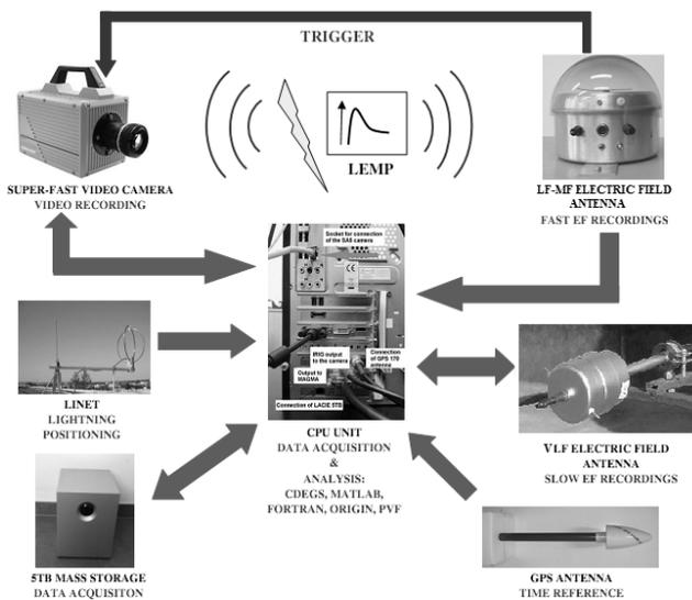
Fig.1. The Lightning Research Station configuration developed at Rzeszow University of Technology.
