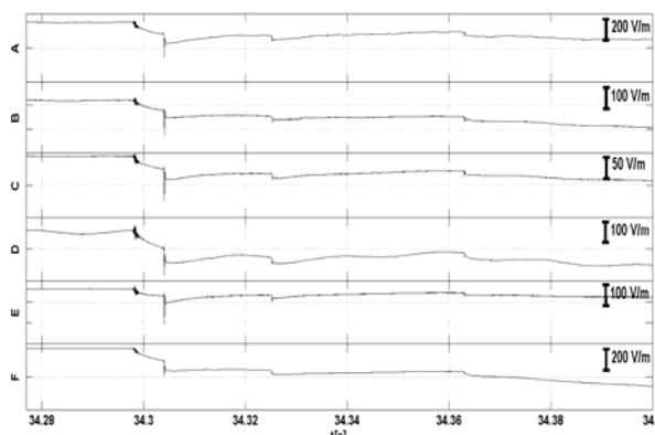
Fig.3. The dedicated LightViewer program showing the same first RS stage of a one multiple CG flash recorded by six various LLDN stations in the Warsaw region.
