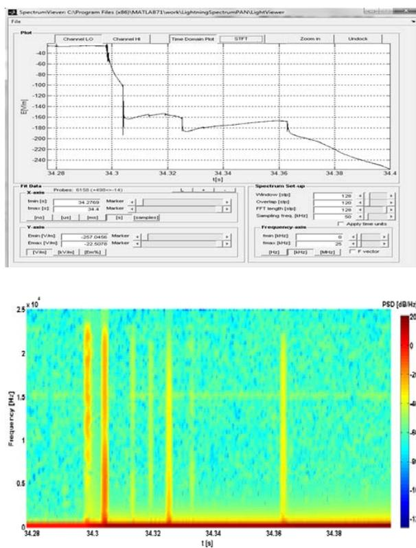
Fig.5. An example of the PSD dynamic spectra analysis used in discrimination of different stroke stages of CG multiple flash. The upper panel – shows a general view of the LightViewer PSD computing interface depicting one of the considered electric field waveforms of multiple CG flash recorded by station F (Fig.3). The bottom panel – gives an example of relevant PSD print-out obtained from the implemented computer data processing.
