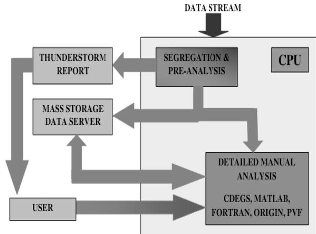
Fig.2. Data acquisition and analysis using dedicated software tools at the Lightning Research Station in Rzeszow.
