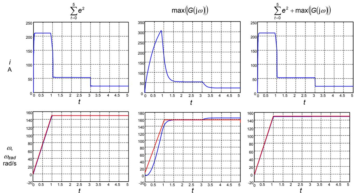
Fig. 8. The armature current and motor speed time-plots obtained during simulation of the motor control system with controllers optimised according to the subsequent quality indices
