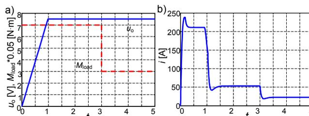
Fig. 3. Time plots of: a) the reference signal  $u_o$  and mechanical torque, b) the armature current
