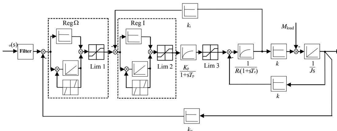
Fig. 2. block diagram of the DC drive system with secondary control loops:  $k_w$  –speed measuring loop gain,  $k_i$  –current measuring loop gain,  $\Omega_o$  - speed reference signal
