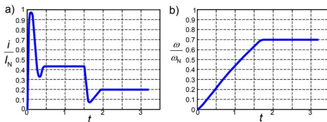
Fig. 12. The motor current (a) and speed (b) after optimisation according to the  $e^2$  criterion
