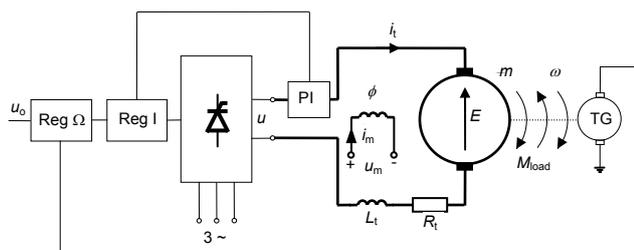
Fig. 1. Schematic diagram of DC drive control with two control loops: PI – current measuring unit; TG – tachogenerator; Reg I – current controller; Reg  $\Omega$  – speed controller
