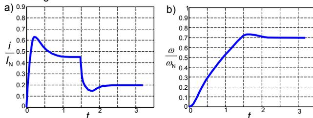
Fig. 14. The motor current (a) and speed (b) after optimisation according to the sum of both norms
