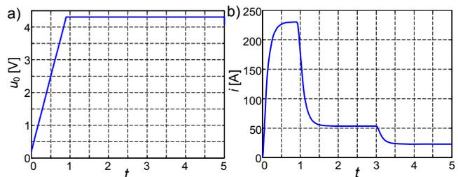
Fig. 6. Time plots of: a) the reference signal  $u_0$ , b) the armature current
