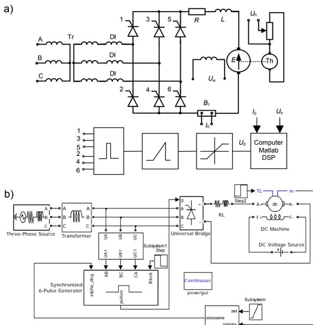
Fig. 10. Diagram of the separately excited motor control system (a) and its Matlab model (b)
