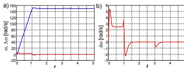
Fig. 4. Time plots of: a) the motor speed signal  $u_o$ , b) the difference between the set and actual motor speed
