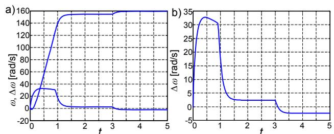
Fig. 7. Time plots of: a) the motor speed signal  $u_0$ , b) the difference between the set and actual motor speed
