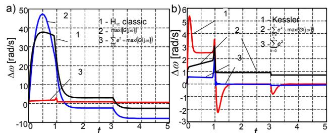
Fig. 9. Summary of the motor speed error optimised according to norms indicated on the plots
