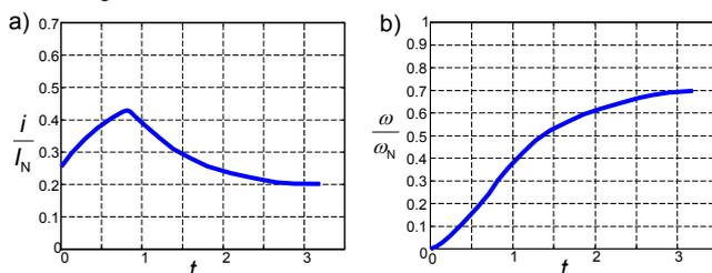
Fig. 13. The motor current (a) and speed (b) after optimisation according to  $H_\infty$  norm
