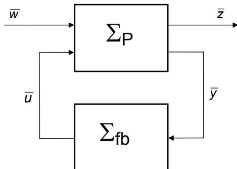
Fig. 5. Basic concept of system controlled according to  $H_\infty$  norm
