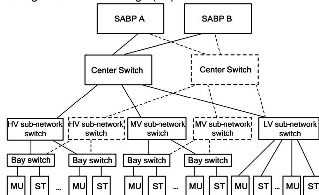
Fig.2. General design of the SABP communication network
