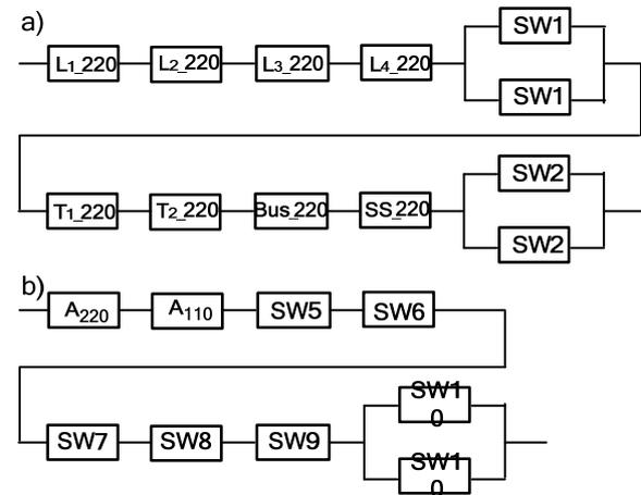
Fig.8. Reliability block diagram of the designed SABP communication network: a) 220kV sub-network, b) whole network.
