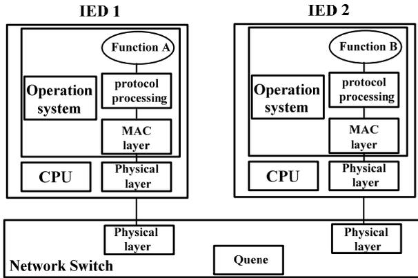
Fig.5. Substation message transmitting procedure.
