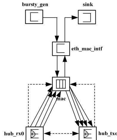
Fig.6. Node model of GOOSE message in OPNET platform.
