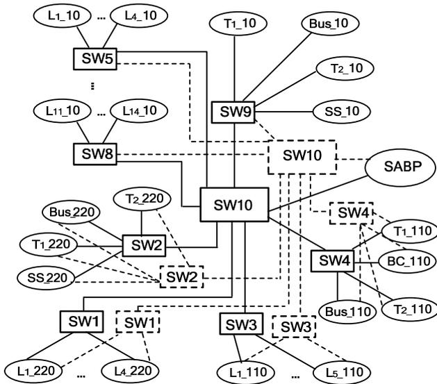
Fig.4. Specific design of the SABP communication network for a practical 220kV smart substation
