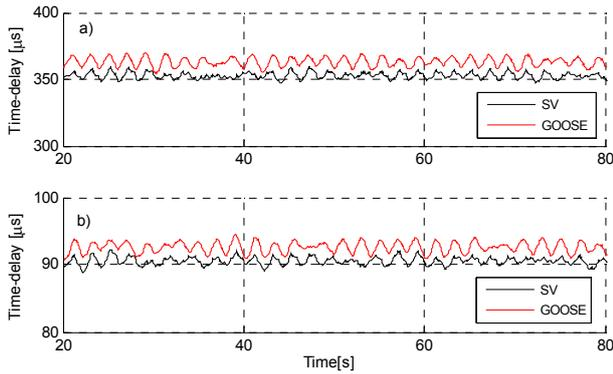
Fig.7. Time-delay simulation characteristics of the networked SV and GOOSE message: (a) without VLAN, (b) with VLAN.
