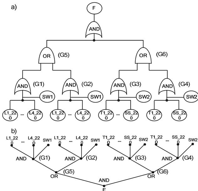
Fig.9. Fault tree and Bayesian model of the 220kV level sub-network: a) fault tree, b) Bayesian model.
