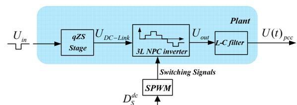
Fig. 2. Open loop block diagram of 3L-NPC qZSI.
