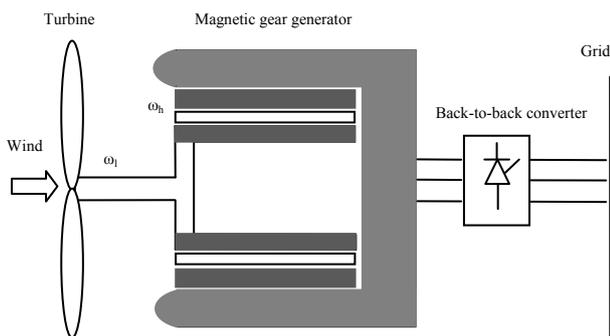
Fig. 4. Magnetic gear generation topology.
