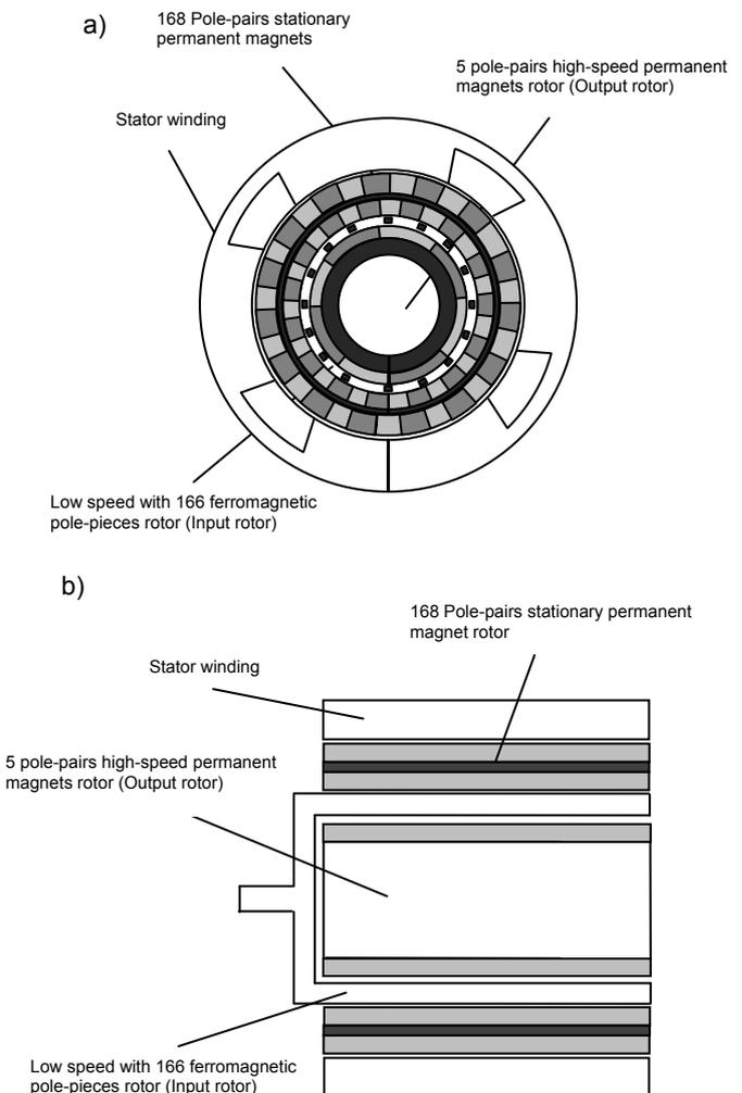
Fig. 1. Magnetic gear generator.
