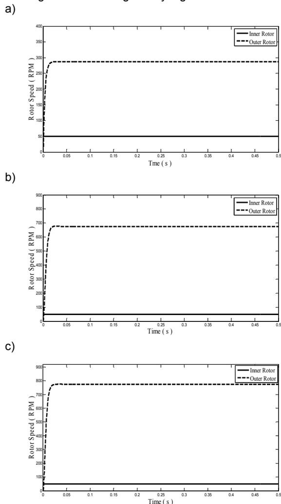
Fig. 3. Standard step response of magnetic gear. (a) For 5.75 gear ratio. (b) For 13.5 gear ratio. (c) For 15.5 gear ratio.
