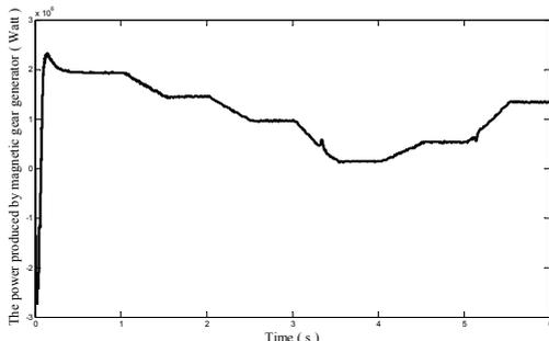
Fig. 9. The power produced by magnetic gear generator.
