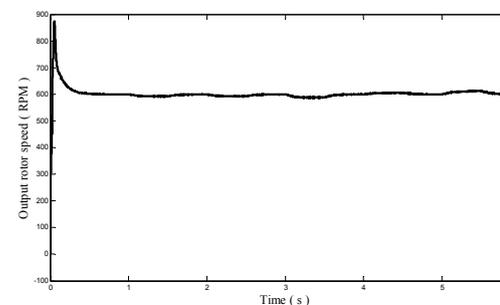
Fig. 7. Rotors speed of the magnetic gear generator
