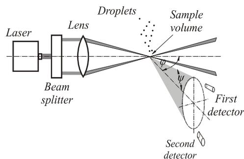
Fig.2. Schematic diagram of a PDPA instrument
