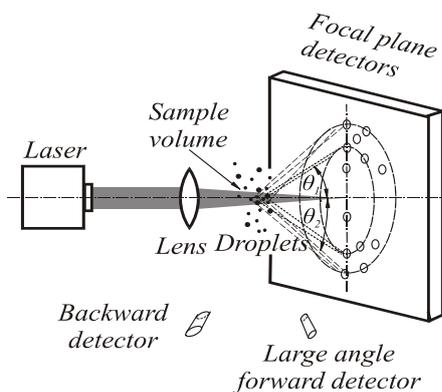
Fig.3. Schematic diagram of an instrument based on the Fraunhofer diffraction technique
