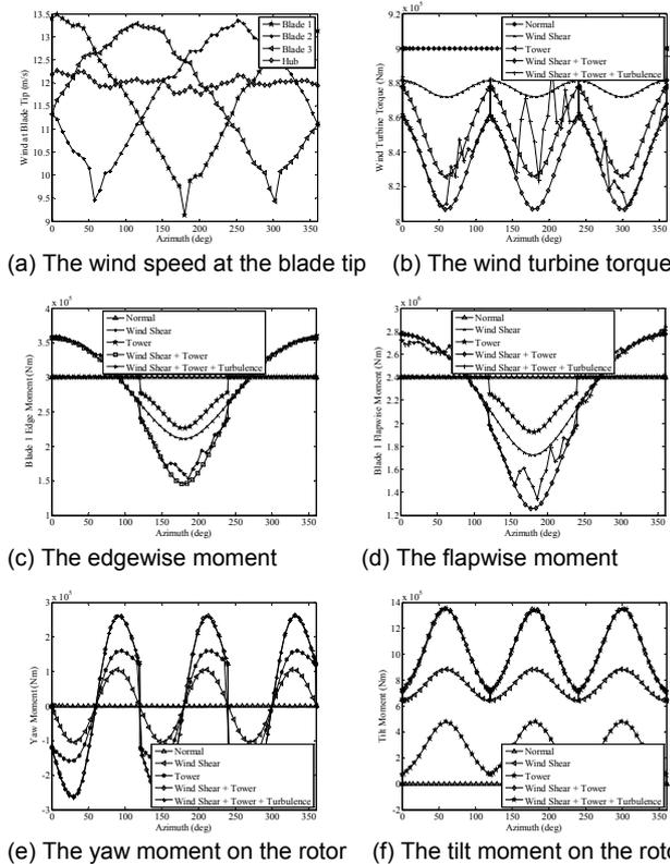
Fig. 2. The loads on the wind turbine affected by wind shear, tower shadow and turbulence
