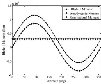
Fig. 1. The relationship diagram of the loads on the blade 1
