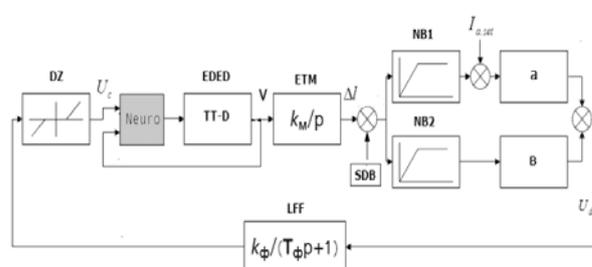
Fig.1. EAF power controller with a neuro-controller functional chart for one phase
