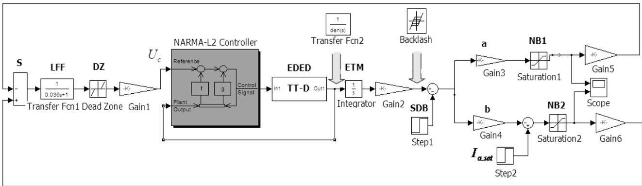
Fig.2. Structural chart of the ARS digital model of EAF-200 arcs lengths
