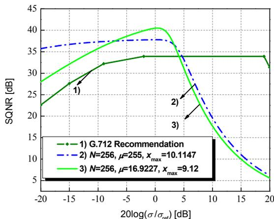
Fig. 1. SQNR characteristics in the wide variance range for  $N = 256$ ,  $\mu = 255$ ,  $x_{\max} = 10.1147$  and  $\mu = 16.9227$ ,  $x_{\max} = 9.12$
