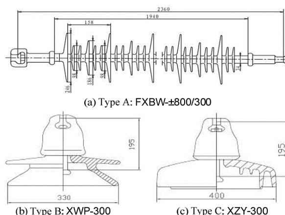
Fig.1. Configuration of the tested insulators
