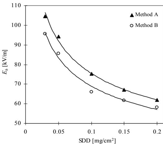
(b) AC flashover voltage gradient of type B insulator string
