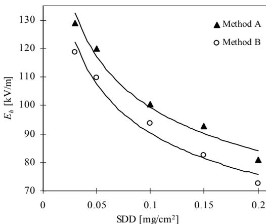
(c) DC flashover voltage gradient of type A insulator
