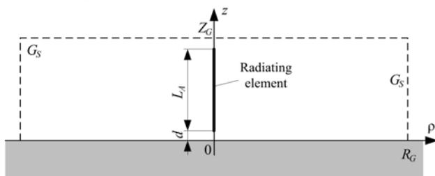
Fig. 1. A circuit of an unbalanced vibrator in the form of a wire antenna
