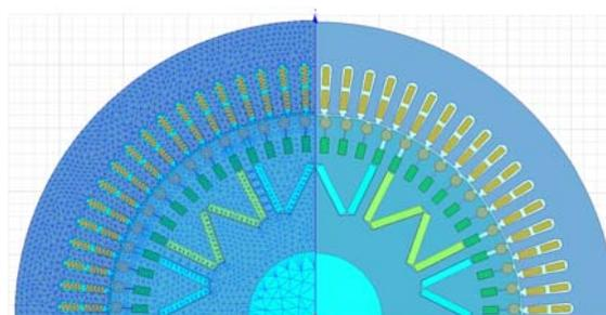
Fig. 1 Field part geometry of the LSPMSM motor model
