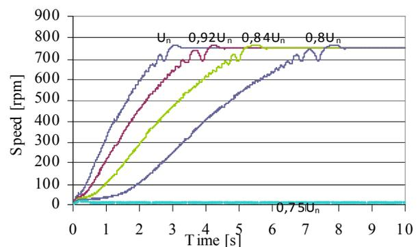
Fig. 5 Transient of rotational speed during motor start for different voltage drops in the supply network.
