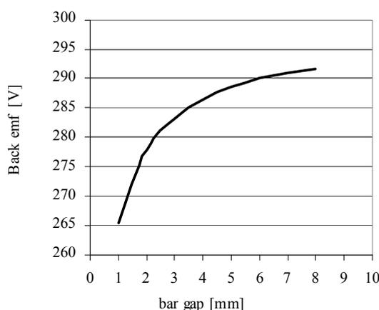
Fig. 2 The effective value of induced voltage depending on the cage bar gap width at the ends of the poles.
