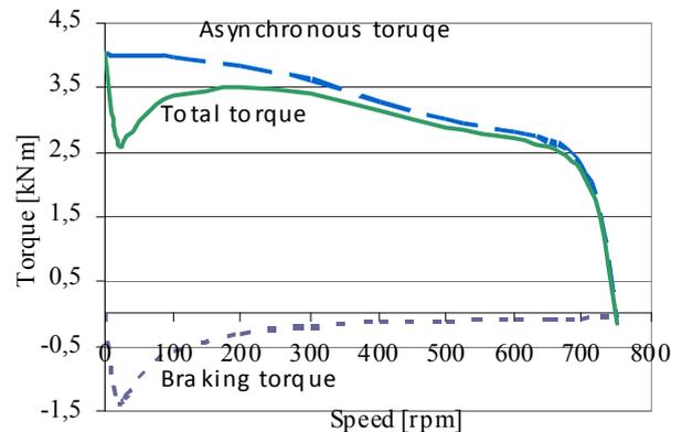
Fig. 4 Total asynchronous torque and its components for the researched LSPMSM motor.
