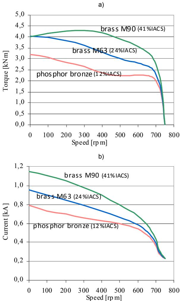
Fig. 3 Asynchronous torque vs. speed (a) and current vs. speed (b) for various starting cage materials.
