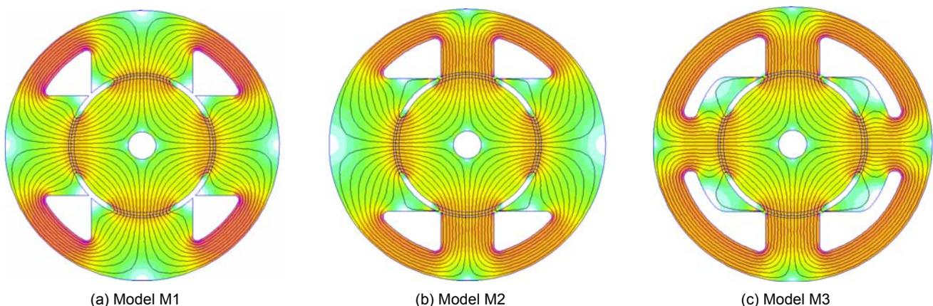
Fig. 4. Field distribution in unexcited BLDCPM motor and 0° rotor position in the derived models M1, M2 and M3
