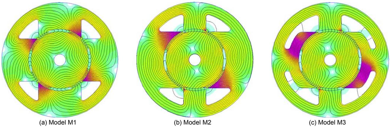
Fig. 5. Field distribution at rated current and 45° rotor position in the derived models of BLDCPM motor M1, M2 and M3
