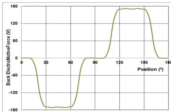
Fig. 11. Back-EMF profile of the motor model M3
