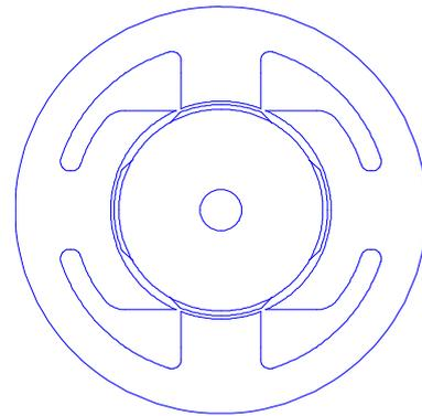
Fig. 3. Shaping the stator poles of BLDCPM motor – M3
