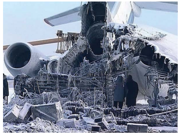
Fig. 21. Tail part of Tu-154B-2 RA-85588 after fire at Surgut airport on January 1, 2011 [2].
