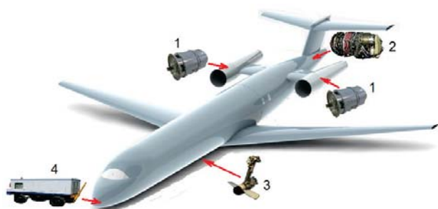
Fig. 1. Aircraft generators: 1 – main generator, 2 – APU, 3 – RAT, 4 – GPU [4].
