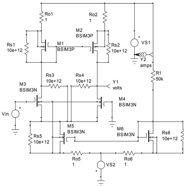
Fig.2. CMOS operational amplifier under test.
