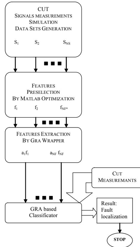
Fig.1. Schematic presentation of diagnostic algorithm using feature preselection and GRA based wrapper.
