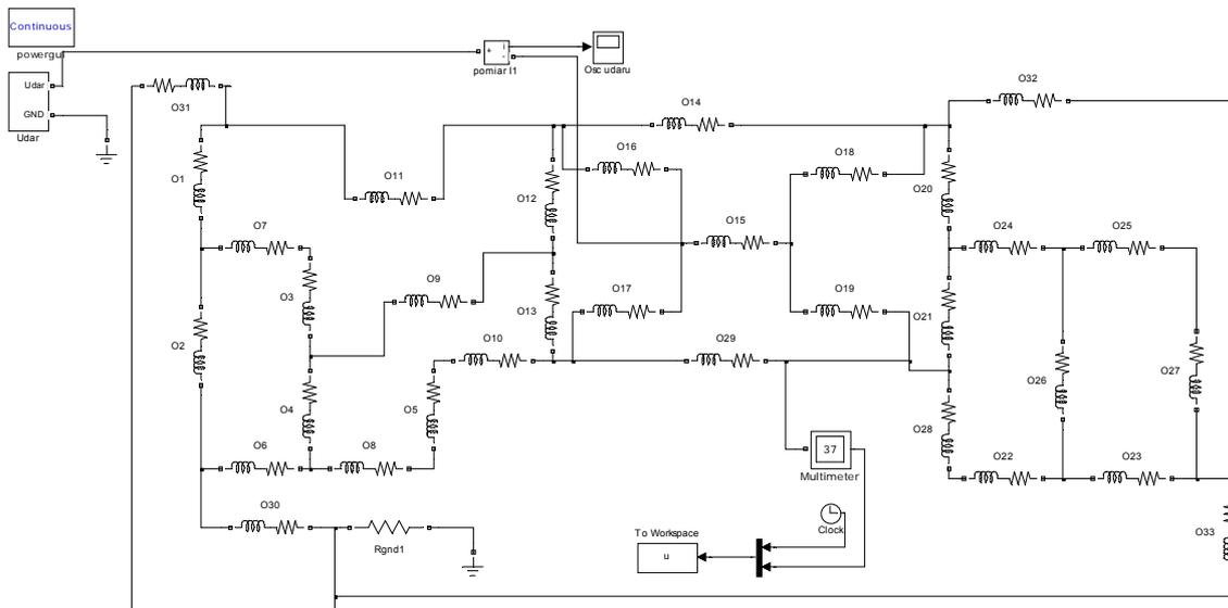
Fig. 2. Simulation model of lightning protection system.
