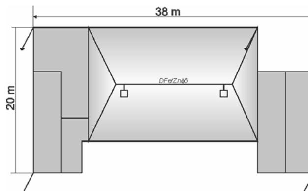
Fig. 1. The plan of the lightning protection system considered object (top view).
